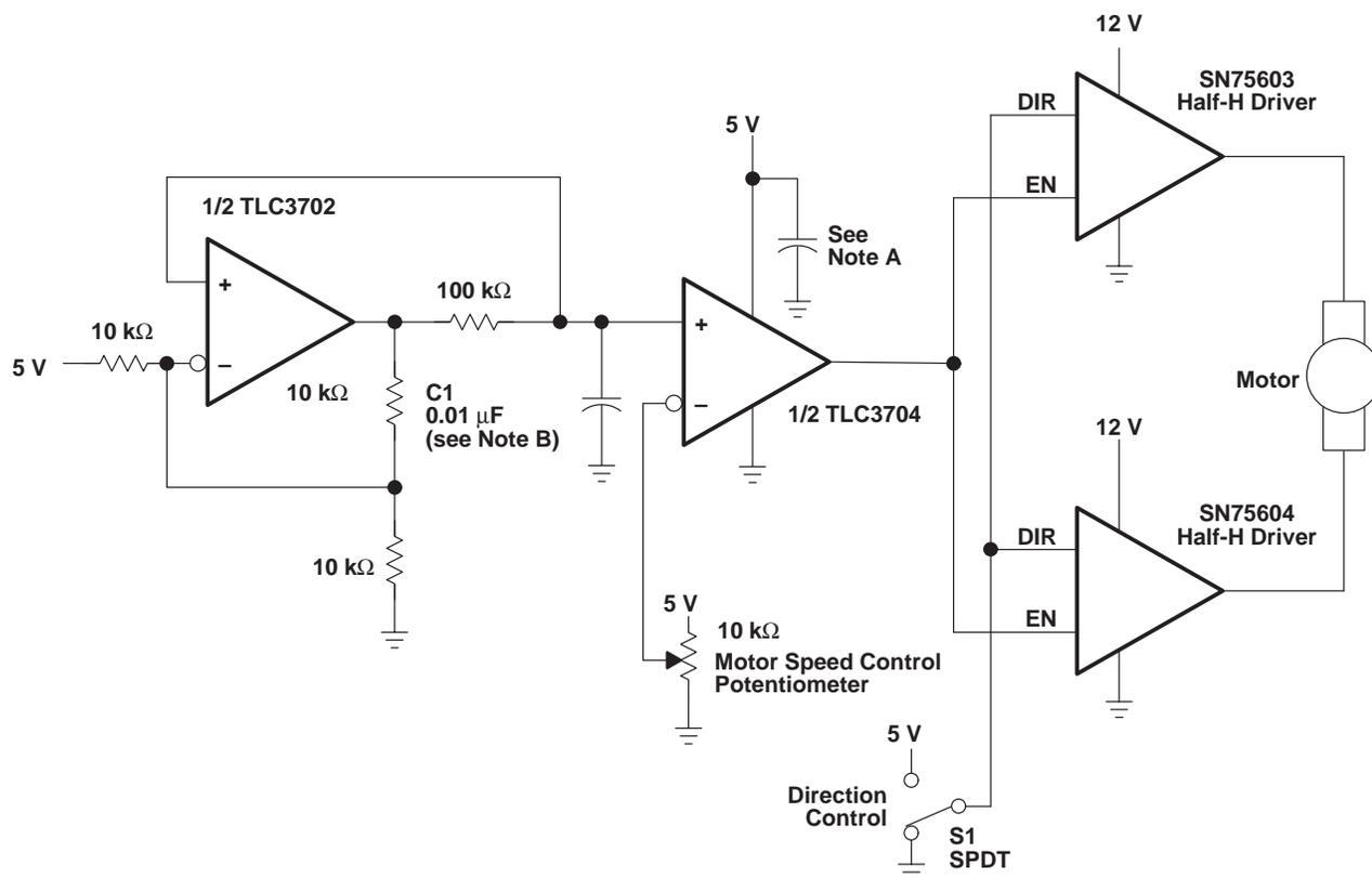
NOTES: A. The recommended minimum capacitance is  $10\text{ }\mu\text{F}$  to eliminate common ground switching noise.
