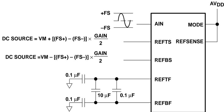
**Figure 19. ADC Reference Generation Mode = AV<sub>DD</sub>**
