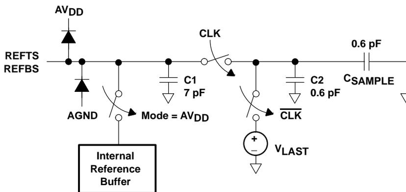
**Figure 37. Equivalent Circuit of REFTS and REFBS Inputs**
