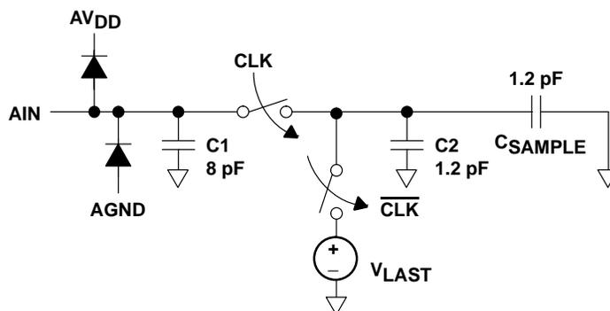
**Figure 32. Equivalent Circuit of Analog Input AIN**
