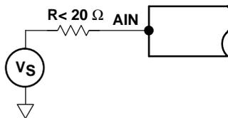
**Figure 33. Damping Source Ringing Using a Small Resistor**
