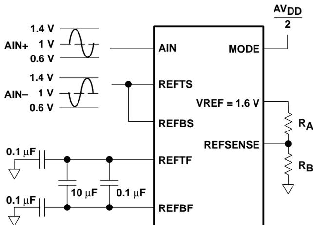
**Figure 25. Differential Operation**
