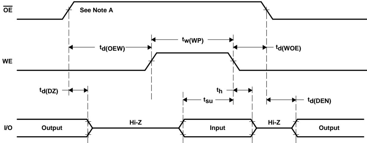
NOTE A: All timing measurements are based on 50% of edge transition.
