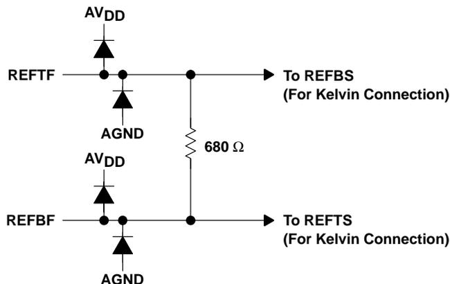
**Figure 38. Equivalent Circuit of REFTF and REFBF Inputs**
