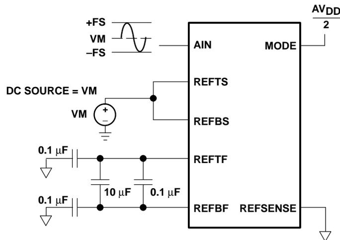
**Figure 17. Center Span Mode, 2-V Reference Span**
