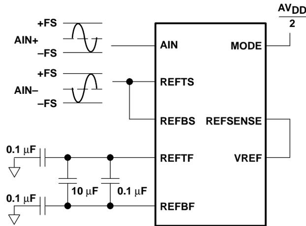
**Figure 16. Differential Input Mode, 1-V Reference Span**
