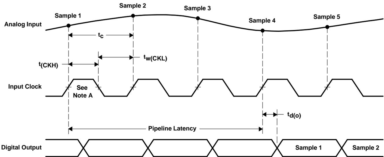
NOTE A: All timing measurements are based on 50% of edge transition.
