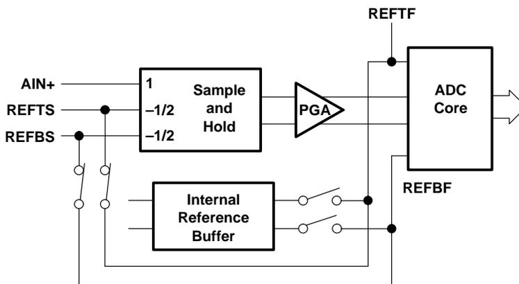
**Figure 12. ADC Reference Generation, MODE = AGND**
