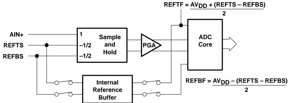
**Figure 18. ADC Reference Generation Mode = AV<sub>DD</sub>**
