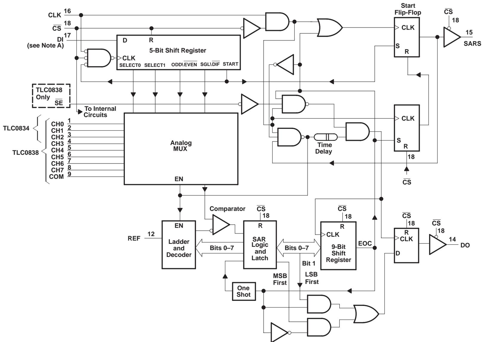
NOTES A: For the TLC0834, DI is input directly to the D input of SELECT1; SELECT0 is forced to a high.
