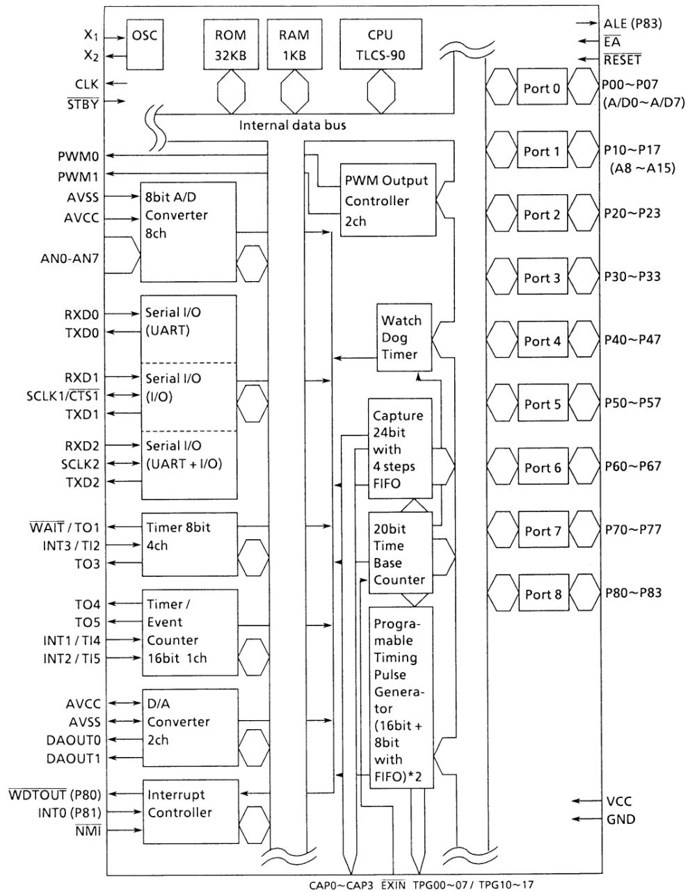
Figure 1. TMP90PM36 Block Diagram
