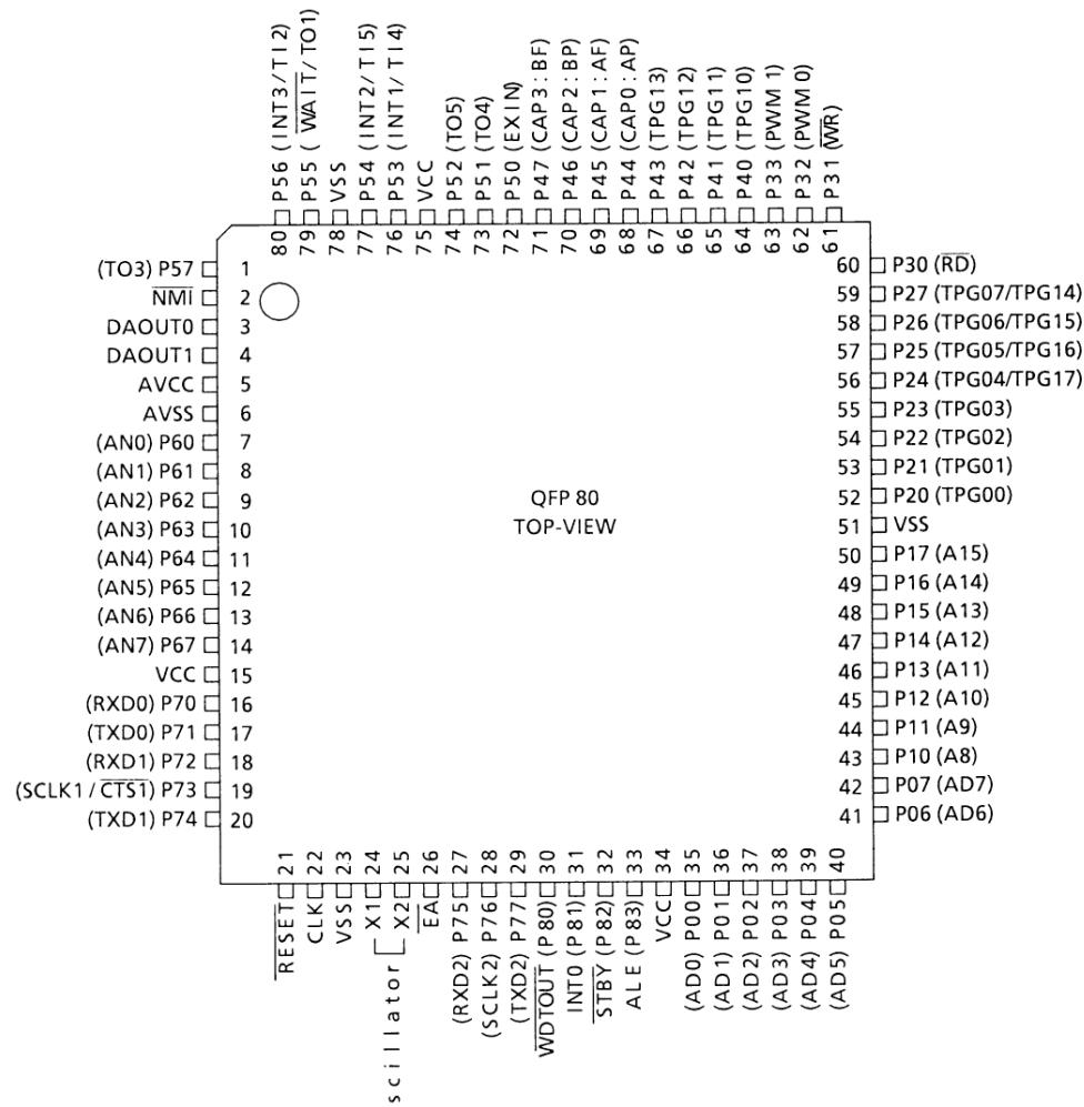
Figure 2.1 (1). Pin Assignments (Flat Package)
