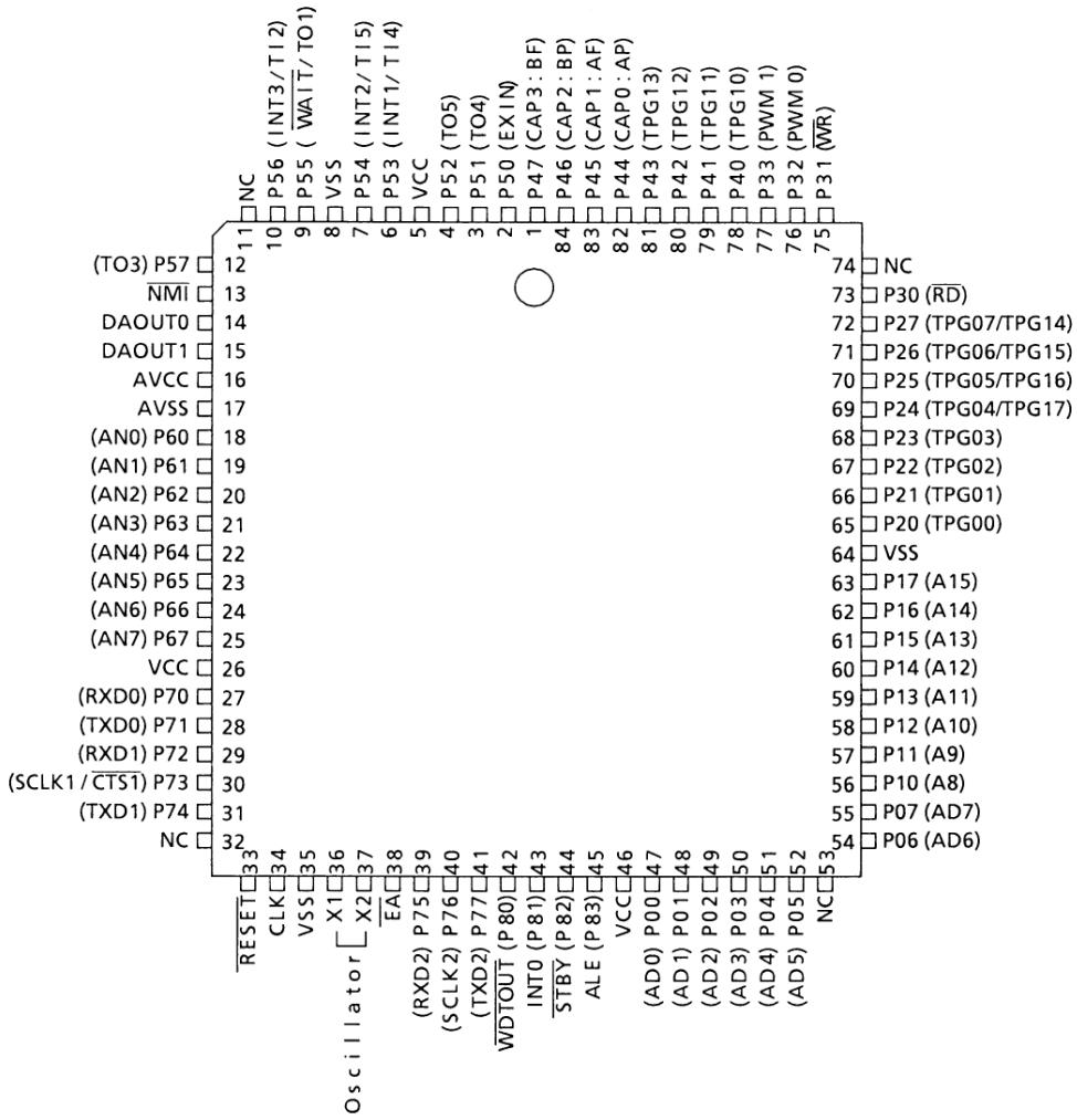
Figure 2.1 (2). Pin Assignments (QFJ (PLCC) Package)
