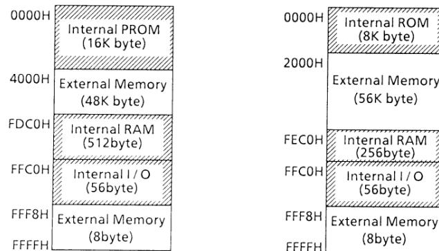
**Figure 1.1. TMP90PH44****Figure 1.2. TMP90C844**
