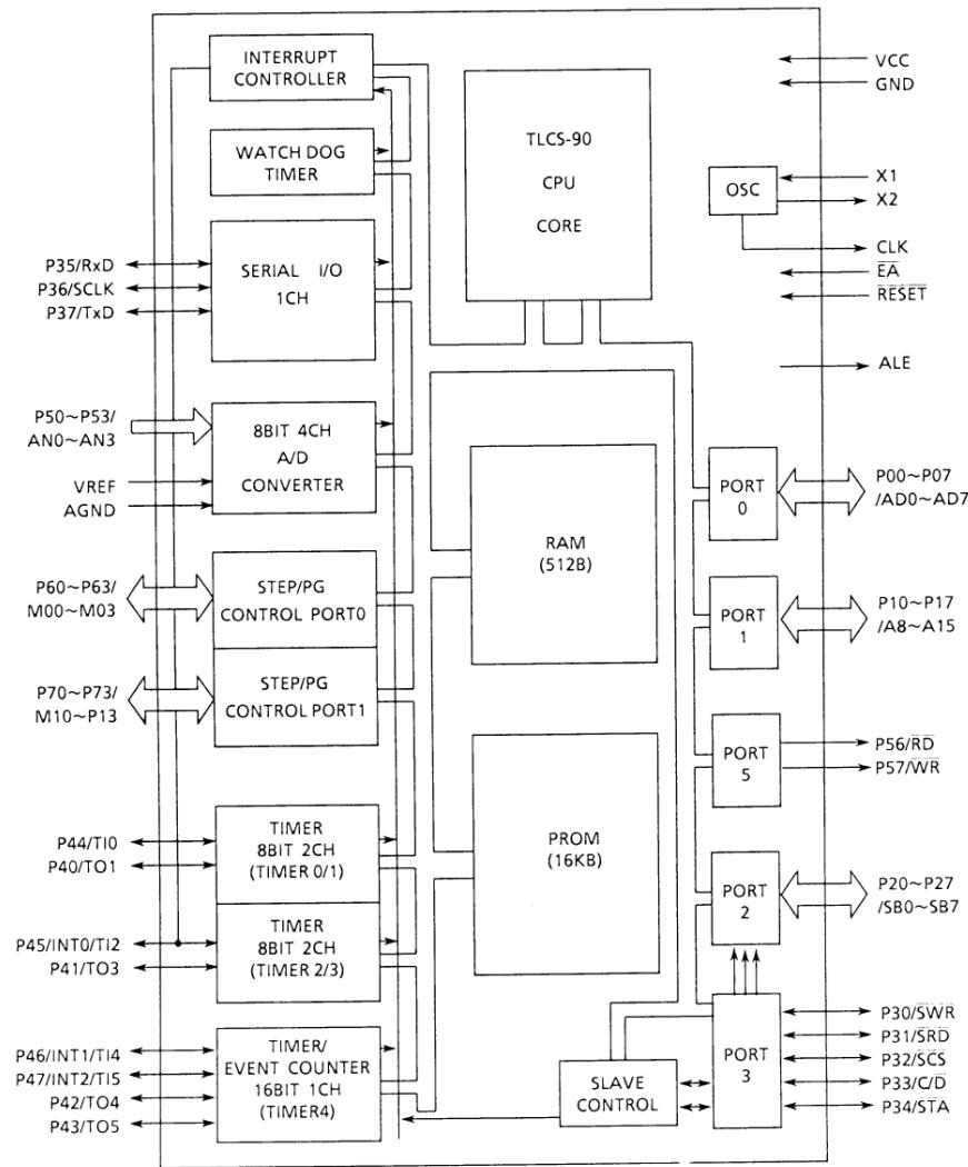
Figure 1.3. TMP90PH44 Block Diagram
