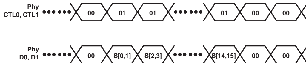
Figure 6. Status Transfer Timing
