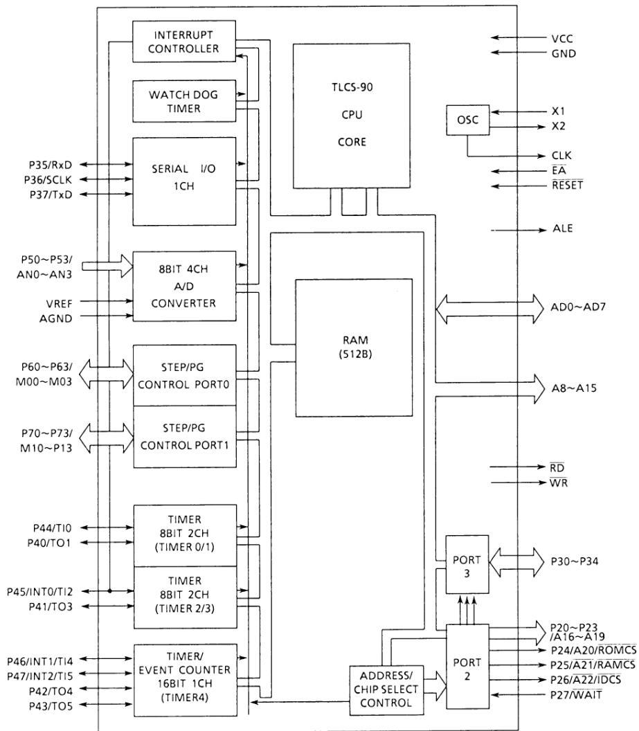
Figure 1. TMP90CH45 Block Diagram
