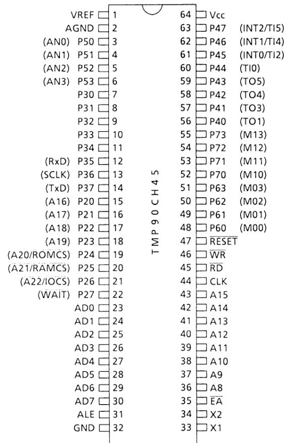
Figure 2.1 (1). Pin Assignment (Shrink DIP)
