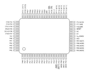
Figure 2.1 (2). Pin Assignment (Flat Package)
