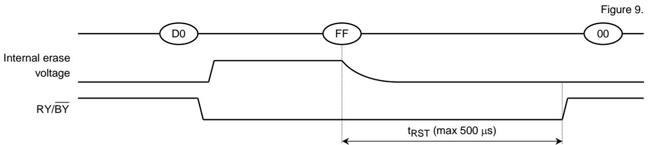
When a Reset (FFH) command is input during Read operation
