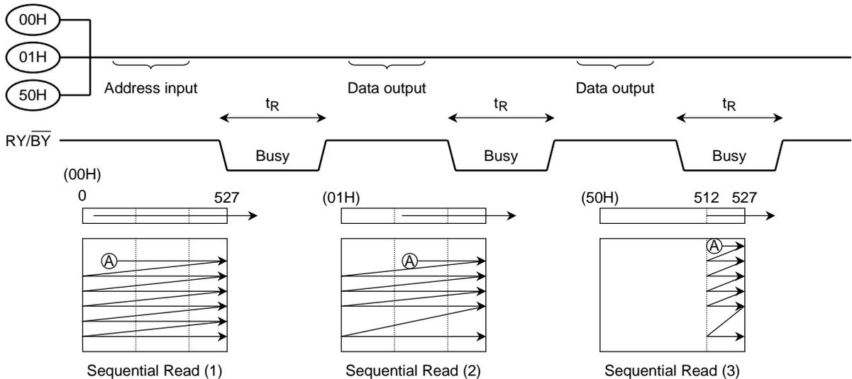
Sequential Read modes (1) and (2) output the contents of addresses 0~527 as shown above, while Sequential Read mode (3) outputs the contents of the redundant address locations only. When the pointer reaches the last address, the device continues to output the data from this address \*\* on each  $\overline{RE}$  clock signal.
