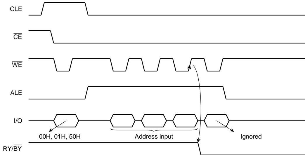
Internal read operation starts when  $\overline{WE}$  goes High in the third cycle.
