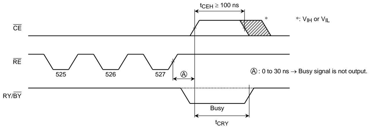
**PROGRAMMING AND ERASING CHARACTERISTICS ( $T_a = 0^\circ$  to  $70^\circ\text{C}$ ,  $V_{CC} = 2.7$  V to 3.6 V)**
