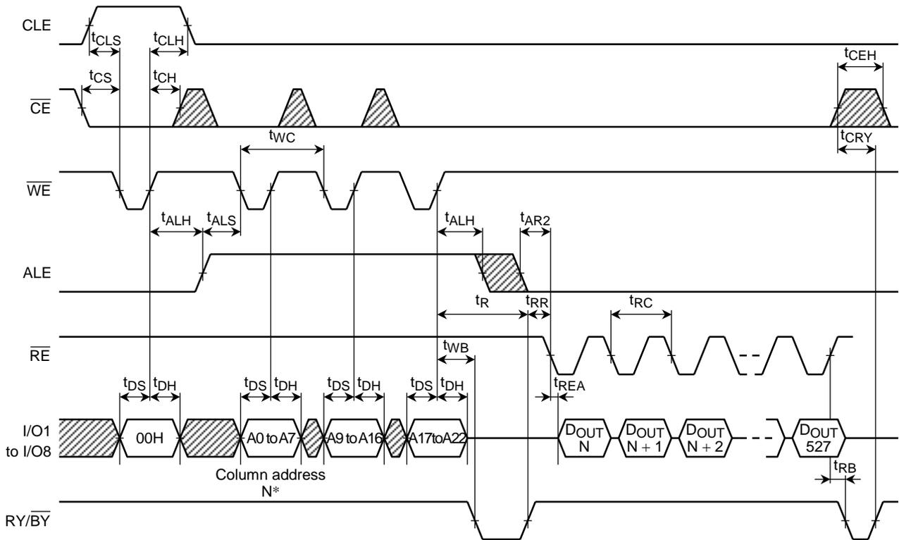
\* Read Operation using 00H Command N: 0 to 255
