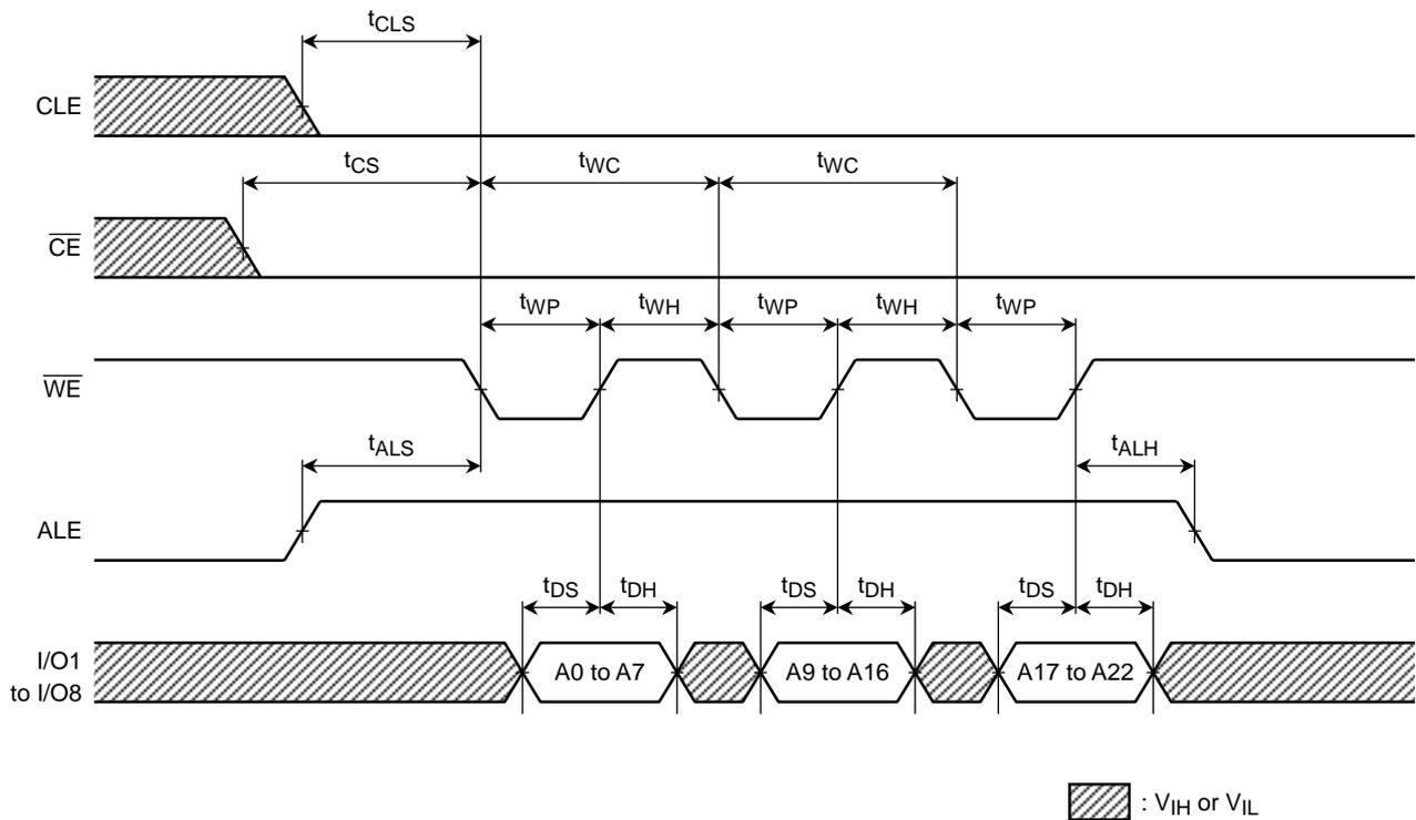
Data Input Cycle Timing Diagram
