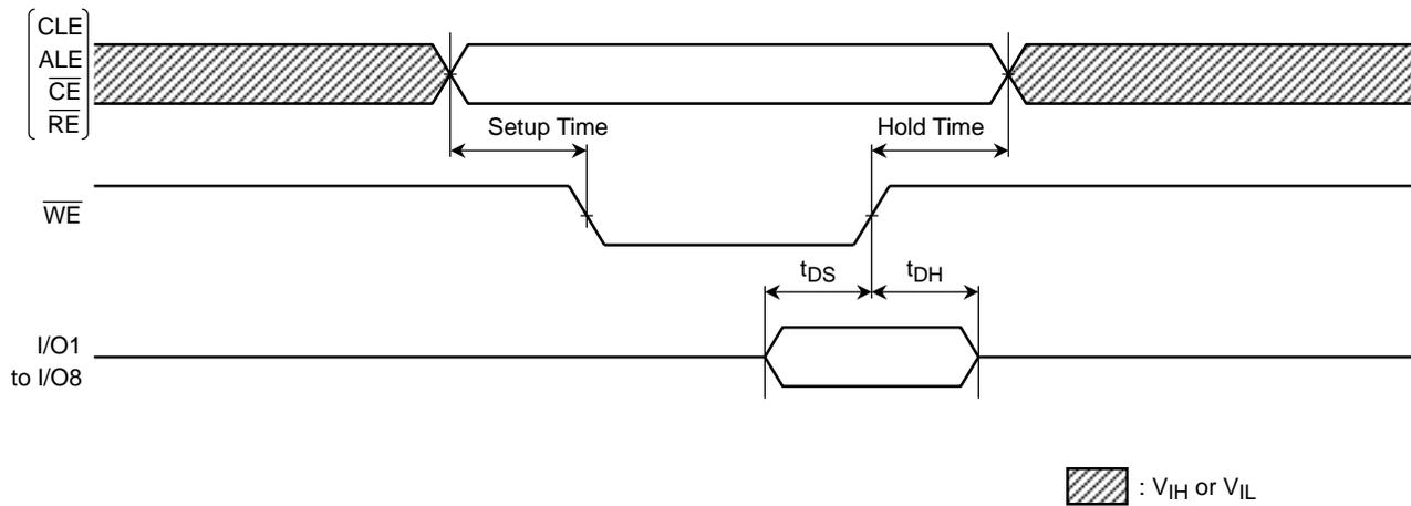
Command Input Cycle Timing Diagram
