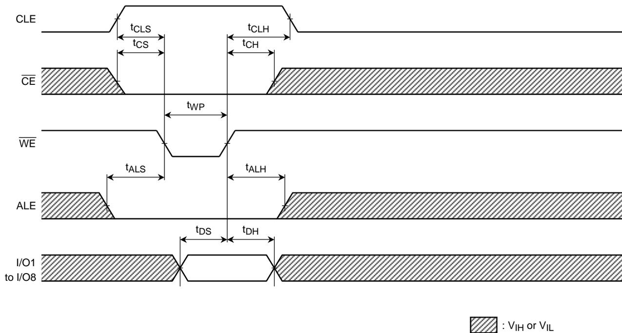
Address Input Cycle Timing Diagram
