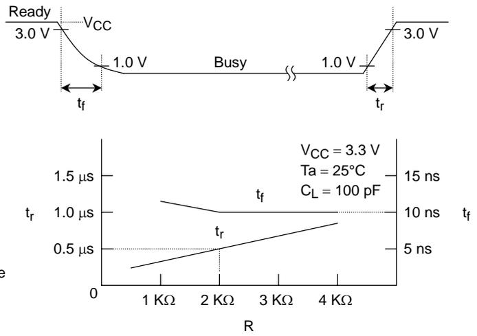
This data may vary from device to device. We recommend that you use this data as a reference when selecting a resistor value.
