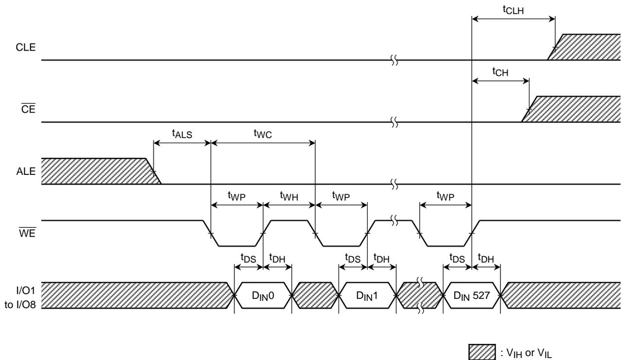
Serial Read Cycle Timing Diagram
