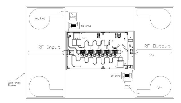
RF connections: Bond using two 1.0-mil diameter, 20 to 25-mil-length gold bondwires at both RF Input and RF Dutput.
