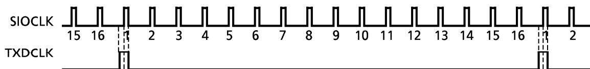
Figure 3.9 (15) Generation of Transmission Clock
