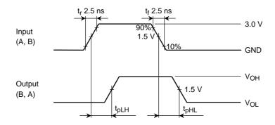
Figure 2 t<sub>pLH</sub>, t<sub>pHL</sub>
