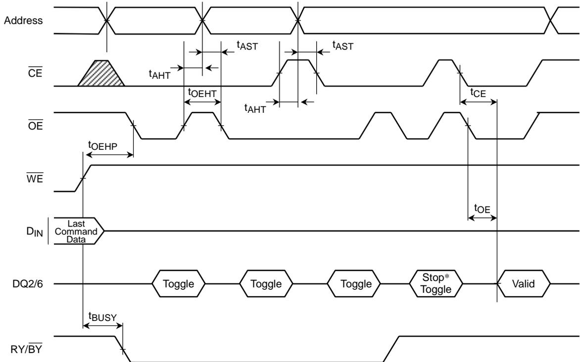
\*DQ2/DQ6 stops toggling when auto operation has been completed.
