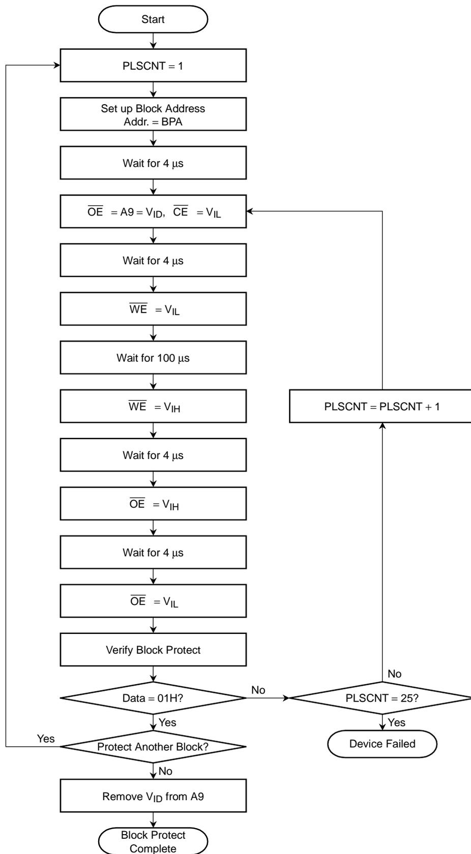
BPA: Block Address and ID Read Address (A6, A1, A0)
