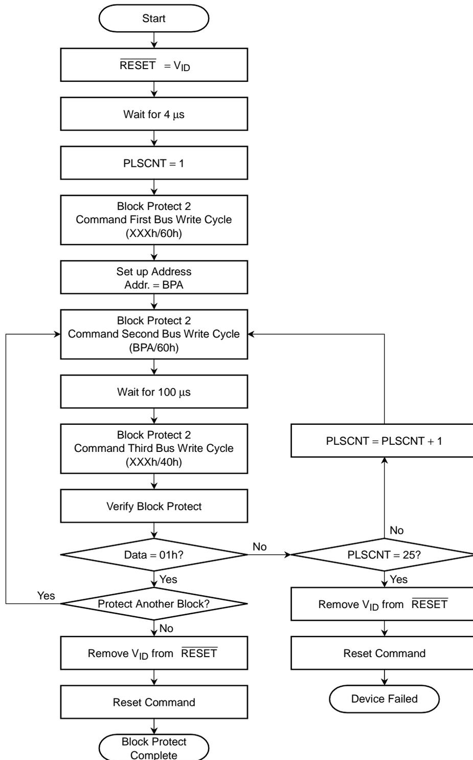
BPA: Block Address and ID Read Address (A6, A1, A0)
