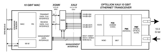
Figure 2 – System connection environment for TOP 3010-LC.
