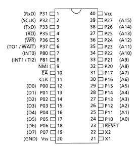
Figure 2.1 (1). Pin Assignment (Shrink Dual Inline Package)
