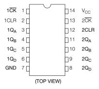
The TC74AC393 is an advanced high speed CMOS DUAL BINARY COUNTER fabricated with silicon gate and double-laver metal wiring C<sup>2</sup>MOS technology.
