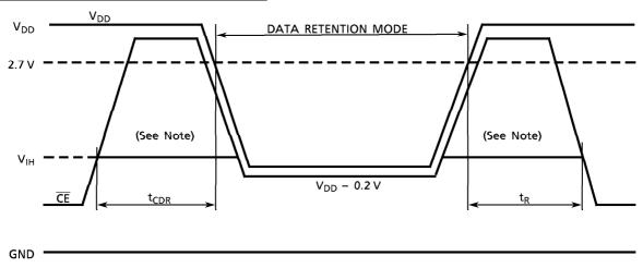
Note: When  $\overline{CE}$  is operating at the  $V_{IH}$  level (2.2 V), the operating current is given by  $I_{DDS1}$  during the transition of  $V_{DD}$  from 3.6 to 2.4 V.
