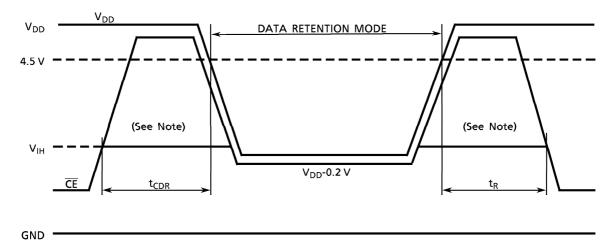
Note: When  $\overline{CE}$  is operating at the  $V_{IH}$  level (2.2V), the standby current is given by  $I_{DDS1}$  during the transition of  $V_{DD}$  from 4.5 to 2.4V.
