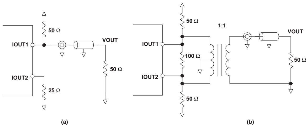
Figure 25. Driving a Doubly Terminated 50 Ω Cable
