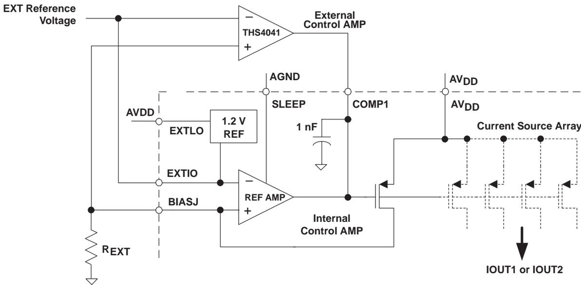
Figure 22. Bypassing the Internal Reference and Control Amplifier
