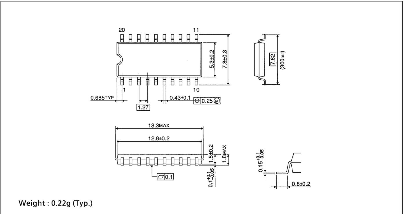
**SOP 20PIN (300mil BODY) PACKAGE DIMENSIONS (SOL20-P-300-1.27)**
