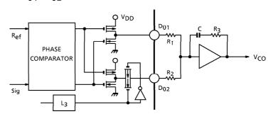
When change a channel, ON the  $D_{02}$  output and make the time constant of the low pass filter smaller to make PLL lock state fastly.
