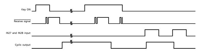
Cyclic pulses are inverted each time a one-shot signal is received.
