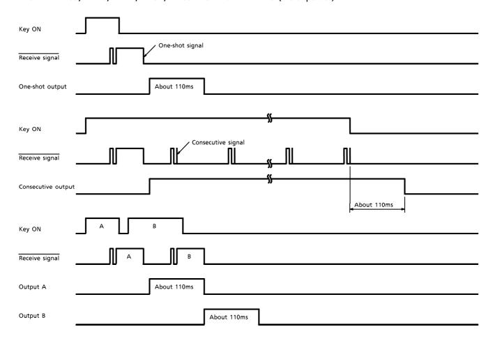
When the initial one-shot system code and the receive signal are checked and the data are valid, the hold pulse is switched to "H" level.
