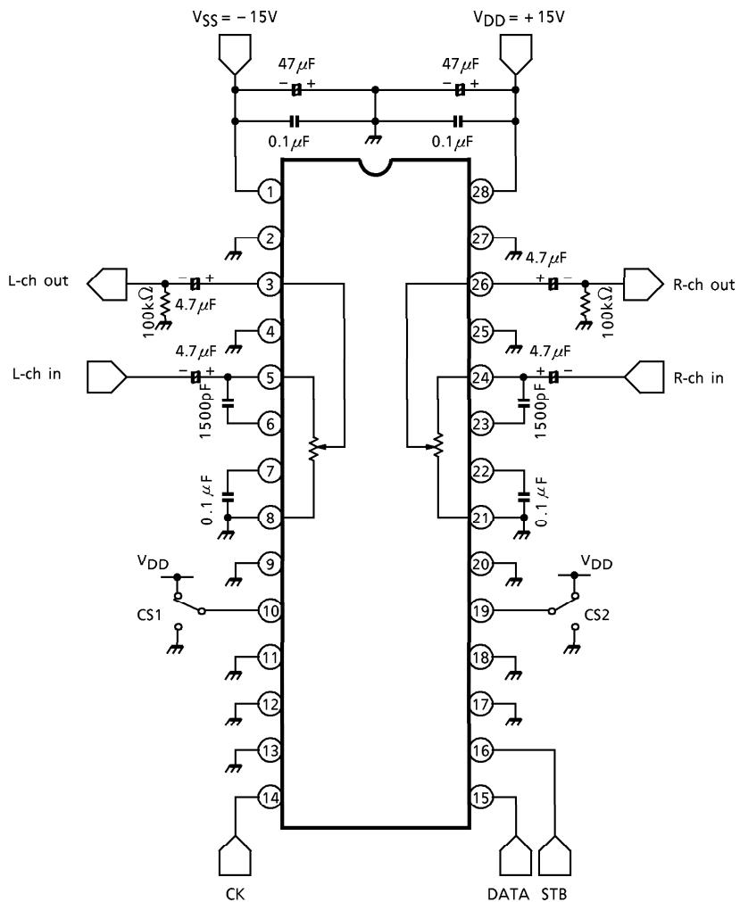
(Note) Since a high-frequency digital signal is input to the CK, DATA and STB pins, corrective measures must be taken to prevent it from getting mixed in the analog circuit to generate noise by, for example, guarding the above signal lines with ground patterns or using shielding wire for these lines.
