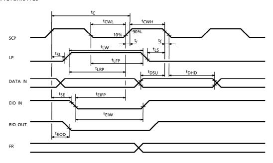
TSET CONDITIONS 1  $(V_{SS} = 0V, V_{DD} = 5V \pm 10\%, V_0 = V_{DD}, V_5 = (V_{DD} - 30) \sim (V_{DD} - 11) V$ , Ta =  $-20 \sim 65^{\circ}$ C)
