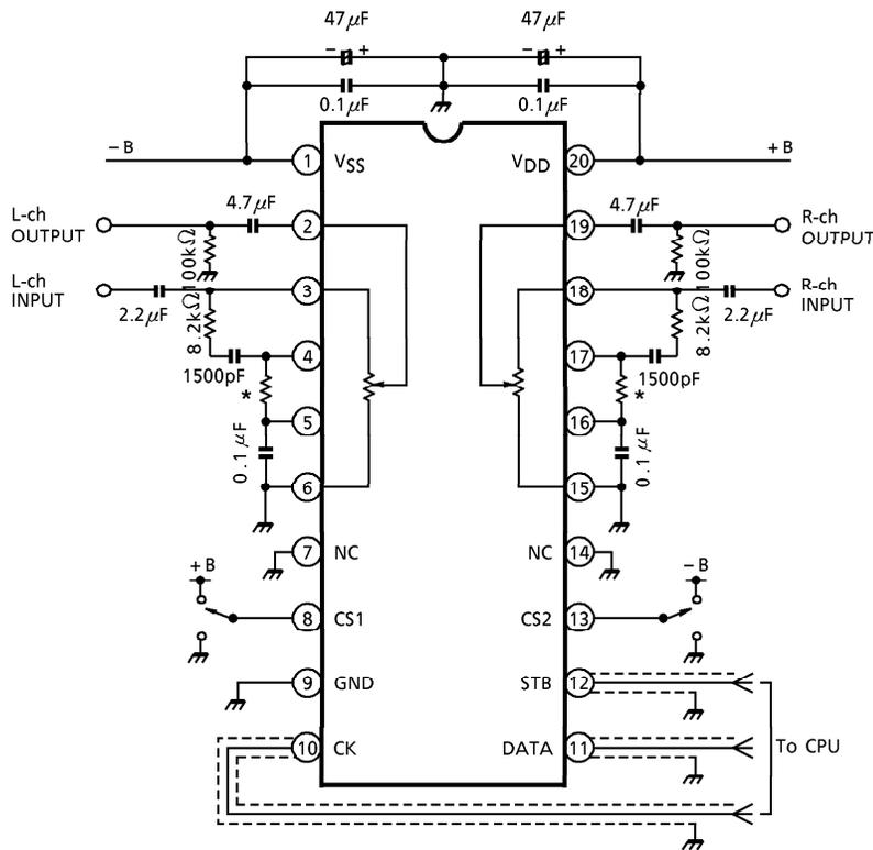
\* Used to prevent noise when loudness control is turned on or off.  $R = 220 \sim 470k\Omega$
