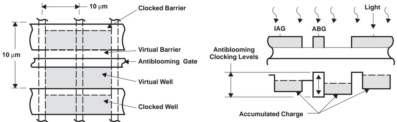
Figure 1. Charge-Accumulation Process
