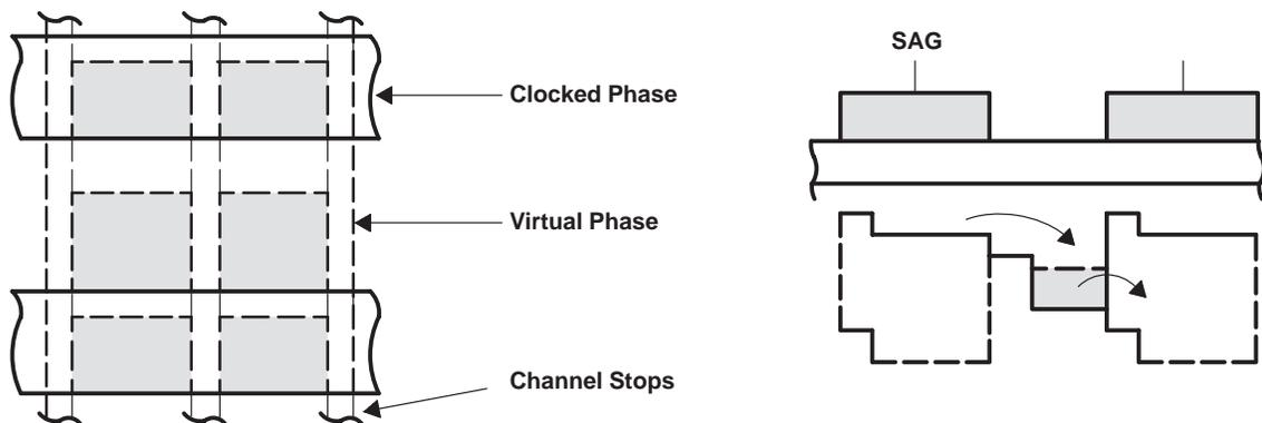
Figure 2. Charge-Transfer Process
