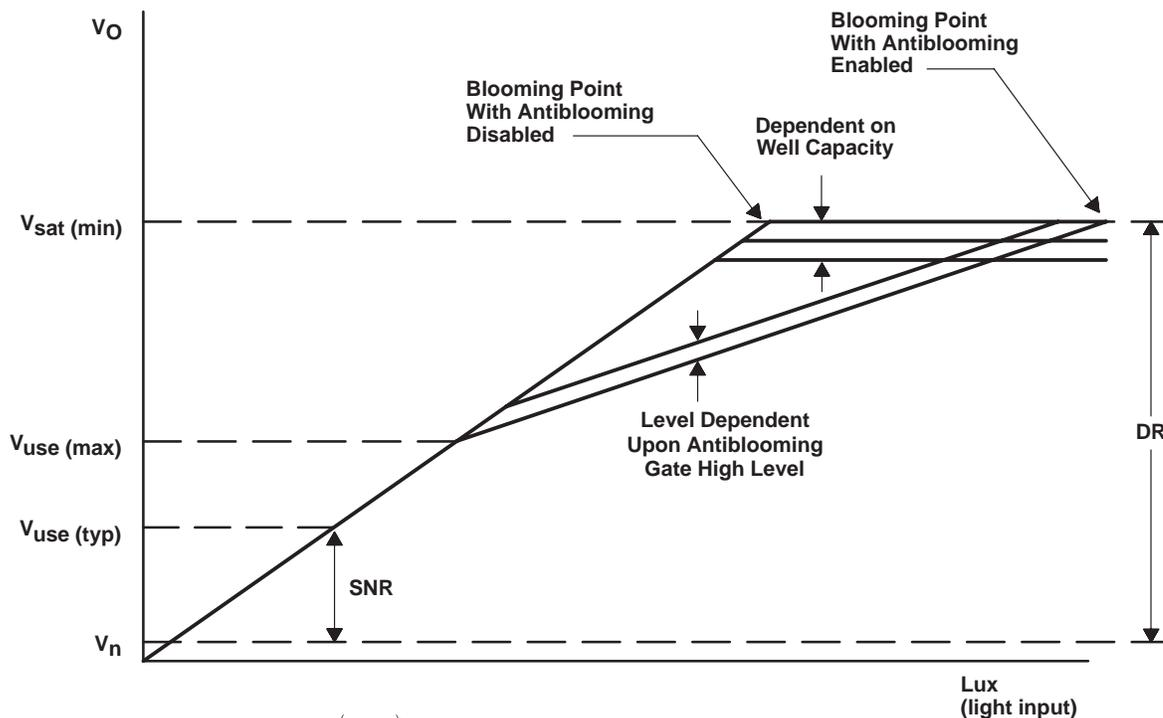
$$DR \text{ (dynamic range)} = 20 \log \frac{(V_{sat})}{V_n} \text{ dB}$$
