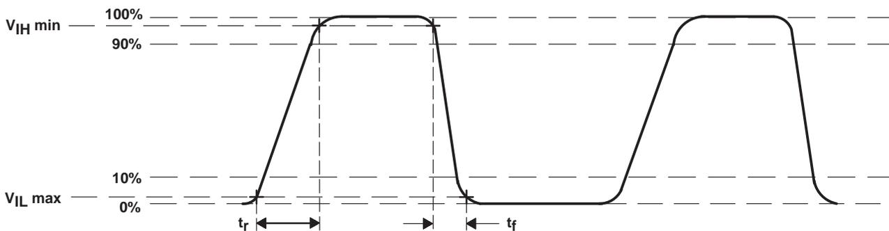
Slew rate between 10% and 90% = 300 V/ $\mu$ s,  $t_r$  =  $t_f$  = 15 ns
