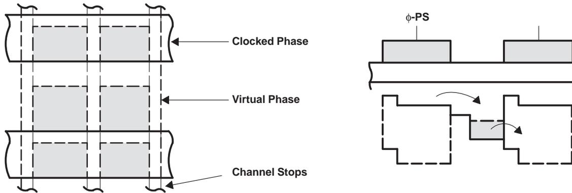
Figure 5. Charge-Transfer Process
