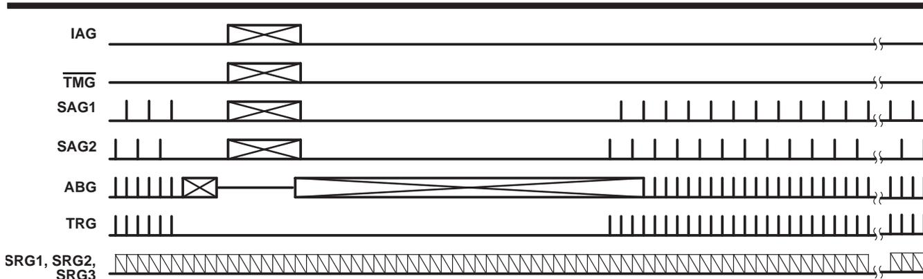
Figure 9. Vertical Timing, Progressive-Scan Mode
