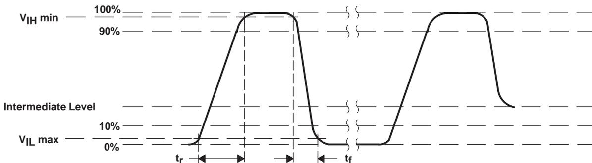
Slew rate between 10% and 90% = 70 to 120 V/ $\mu$ s,  $t_r$  = 150 ns,  $t_f$  = 90 ns
