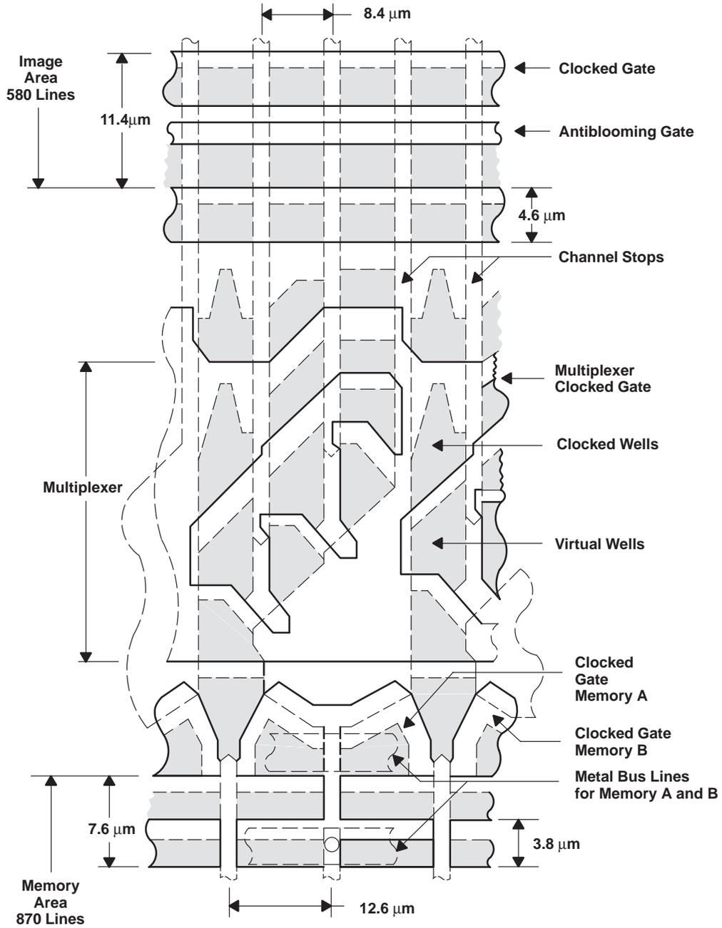
Figure 1. Layout of Multiplexing Gate
