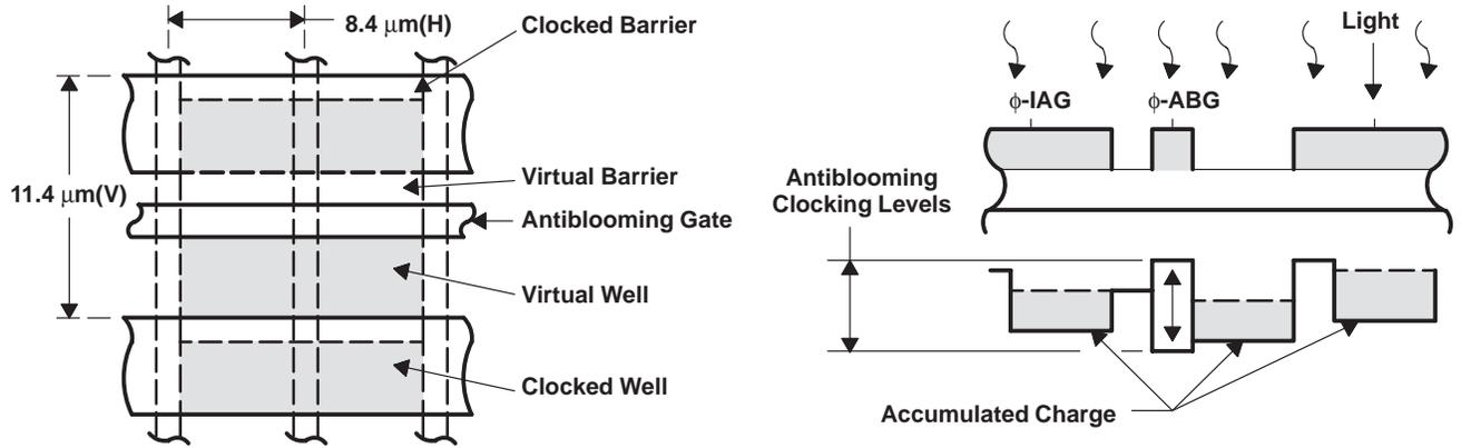
Figure 4. Charge-Accumulation Process
