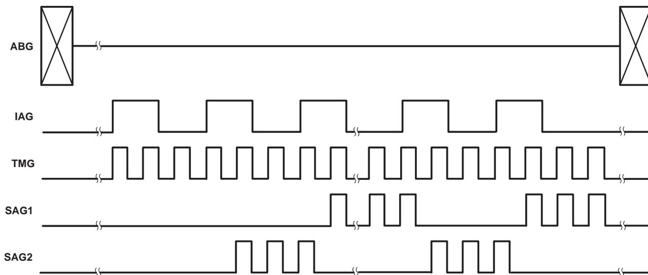
Figure 10. Parallel-Transfer Timing
