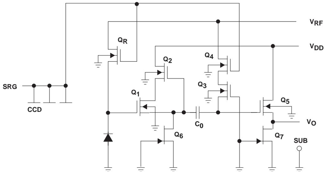
Figure 4. Charge-Detection Schematic
