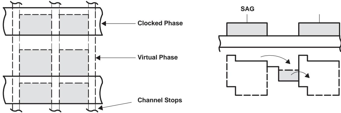
**Figure 2. Charge-Transfer Process**
