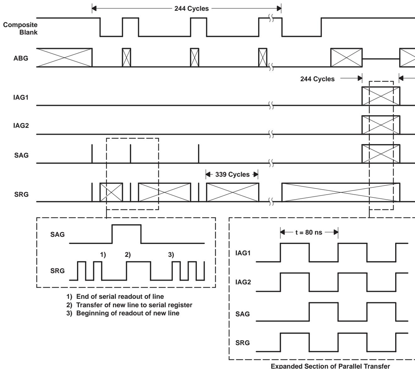
Figure 3. Timing Diagram
