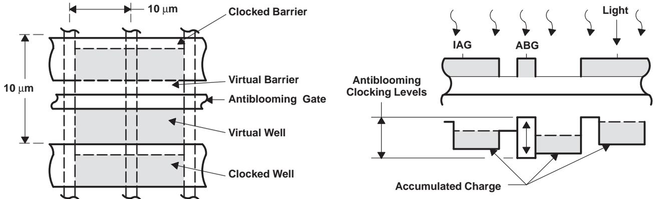
**Figure 1. Charge-Accumulation Process**
