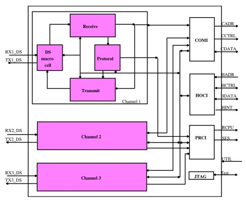
Target applications are heterogeneous multi-processor systems supported by scalable interfaces including the little/big endian swapping. The TSS901E connects modules with different processors (e.g. 21020F, ERC32, TSC695E and others). Any kind of network topology could be realized through the high speed point-to-point IEEE1355-links (see chapter Applications).
