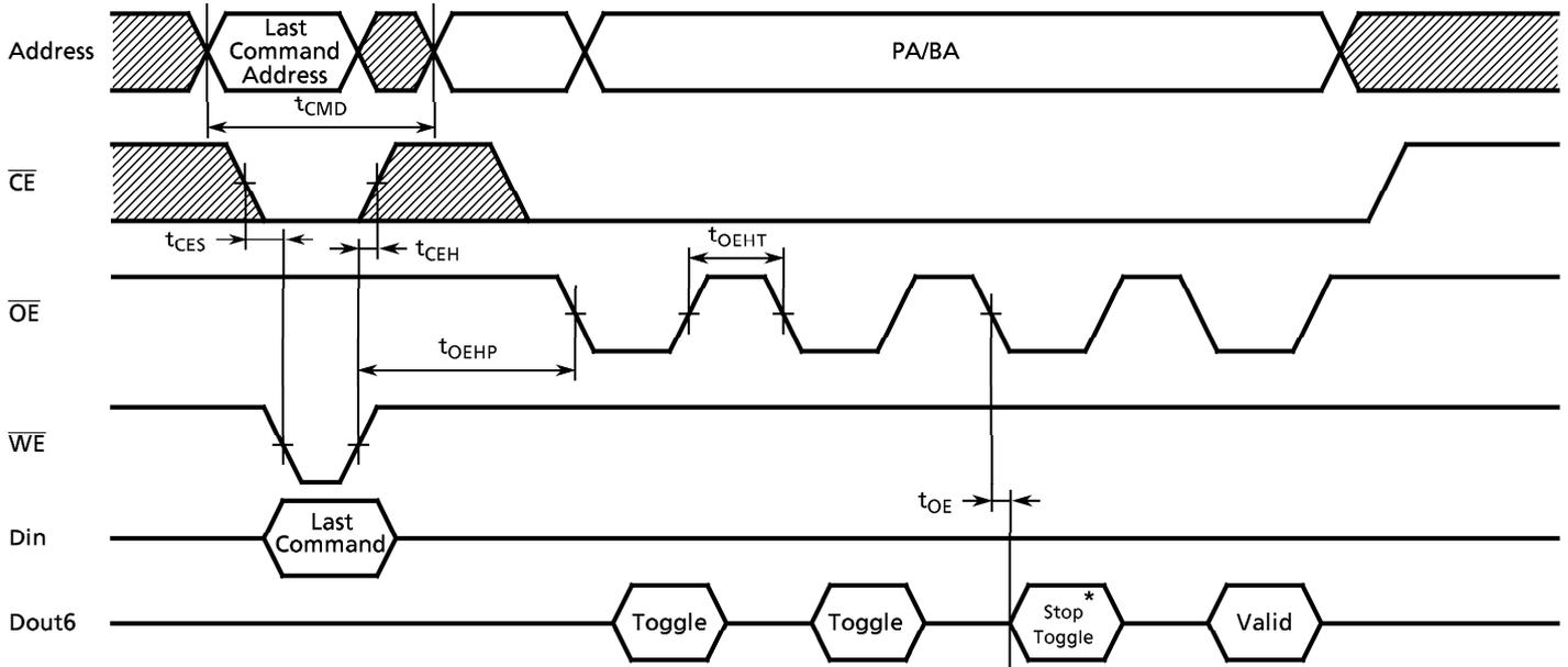
\* Dout6 stops toggling when the last command has completed.
