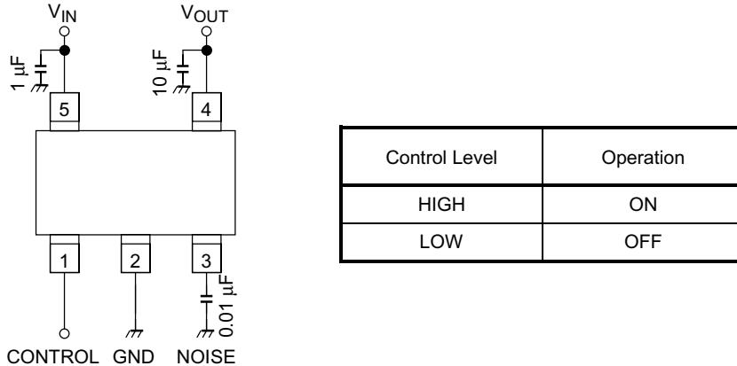
The figure above shows the recommended configuration for using a point regulator. Insert a capacitor for stable input/output operation. If the control function is not to be used, Toshiba recommend that the control pin (pin 1) be connected to the VCC pin.
