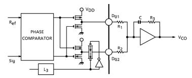
When change a channel, ON the  $D_{02}$  output and make the time constant of the low pass filter smaller to make PLL lock state fastly.
