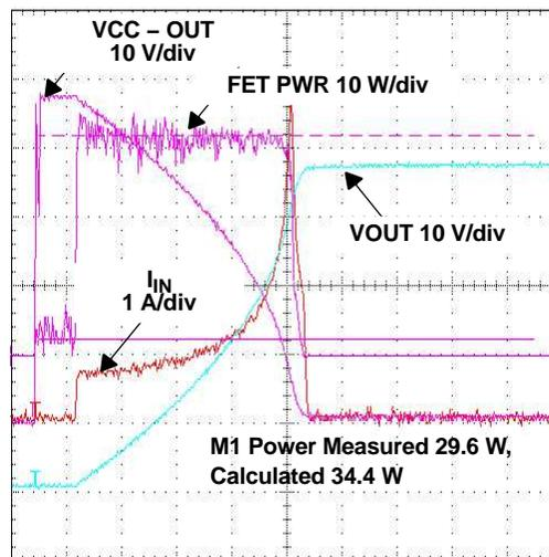
Figure 13. Computation of M1 Stress During Startup
