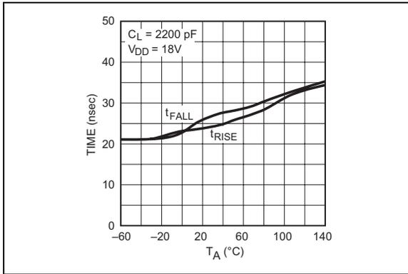
**FIGURE 2-7:** Rise and Fall Times vs. Temperature.
