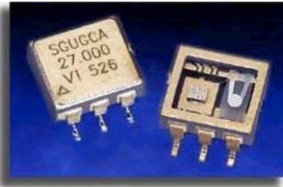
**The S-Type Voltage Controlled Crystal Oscillator**
