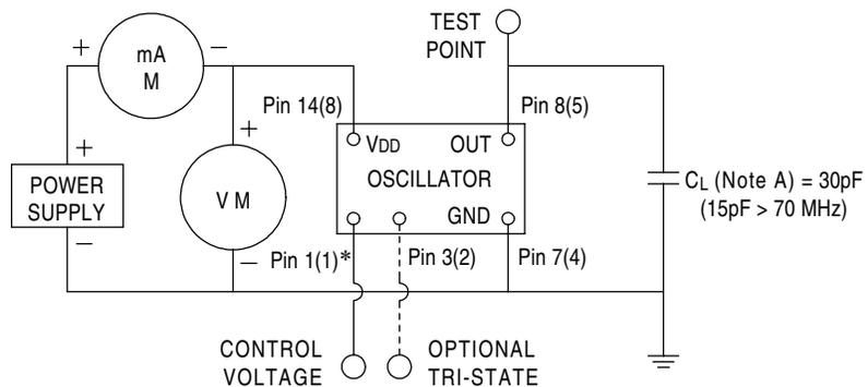
NOTE A: C<sub>L</sub> includes probe and fixture capacitance
