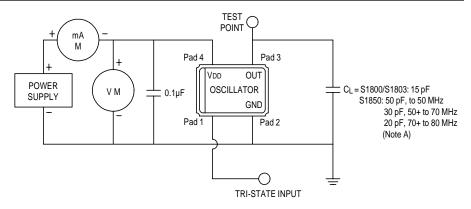
Note A: CL includes probe and fixture capacitance
