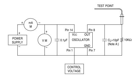
NOTE A: CL includes probe and fixture capacitance.
