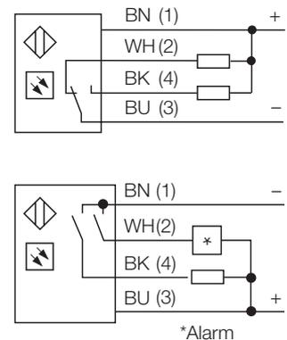
The emitter and receiver are incorporated in a single housing. The light reflection of the target is detected and triggers the sensor to switch. Thus the switching distance depends largely on the reflectivity of the target.
