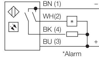
The emitter and receiver are incorporated in a single housing. The light reflection of the target is detected and triggers the sensor to switch. Thus the switching distance depends largely on the reflectivity of the target.
