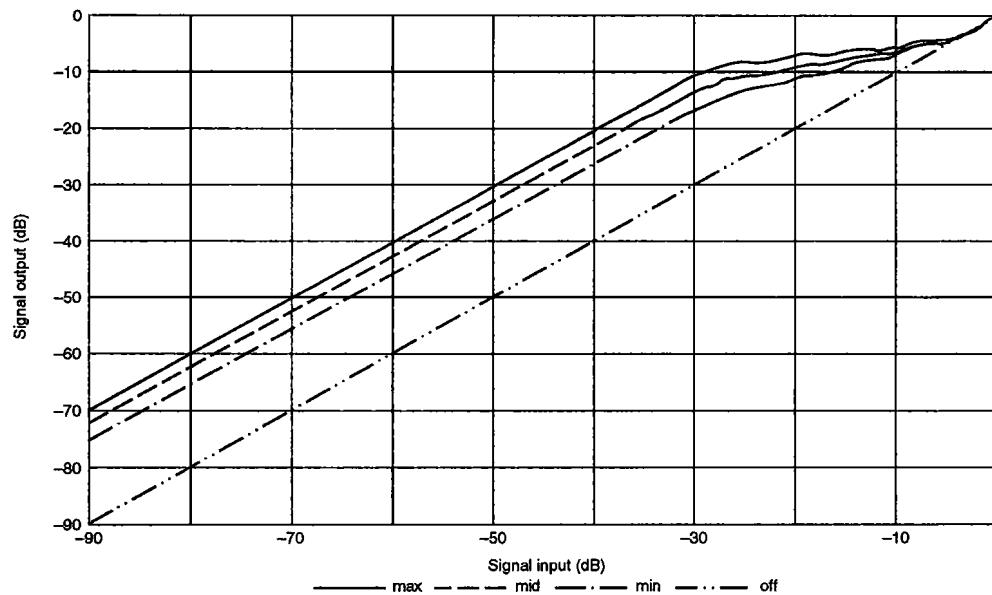
**Input/output gain characteristics**
