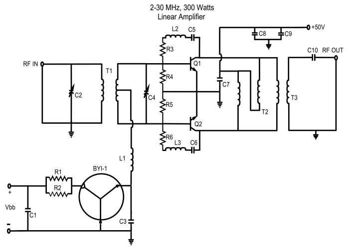
Q1,Q2=Ghz S175-50 BYISTOR=GHz BYI-1 C1,C3,C5,C6,C7,C8=0.1mF ceramic C2=25-240pF Compression Mica C4=75-480pF Compression Mica C9=10mF, 50V, Electrolytic C10=2700pF DM15 L1=6 turns on Indiana General F627-9, H Material L2,L3=2.2mH, Molded Inductor R1,R2=22W, 2 Watts R3,R6=220W, 2 Watts R4,R5=10W, 1/4 Watt
