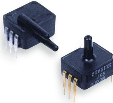
The SDX series sensors provide a very cost effective solution for pressure applications that require small size plus performance. These calibrated and temperature compensated sensors give an accurate and stable output over a 0 °C to 50 °C [32 °F to 122 °F] temperature range. This series is intended for use with non-corrosive, non-ionic working fluids such as air, dry gases and the like.
