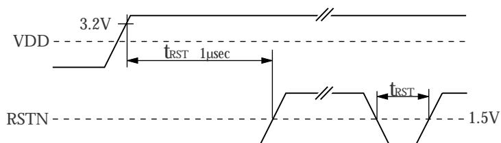
RSTN should be set LOW at power-ON and after reacquiring synchronization. Note that if RSTN is LOW for longer than 1 μs, a through-current flows in the internal dynamic circuits because the internal clock is stopped. The through-current has no rated value, so the reset pulse should be kept as short as possible at all times other than at power-ON.
