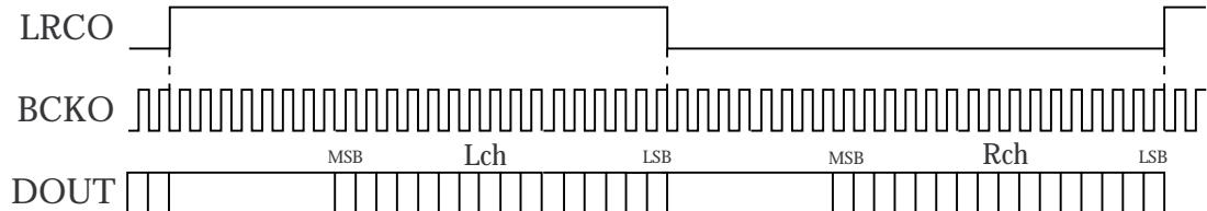
There must be a minimum of 16 BCKI clock cycles to read in a single word of data.
