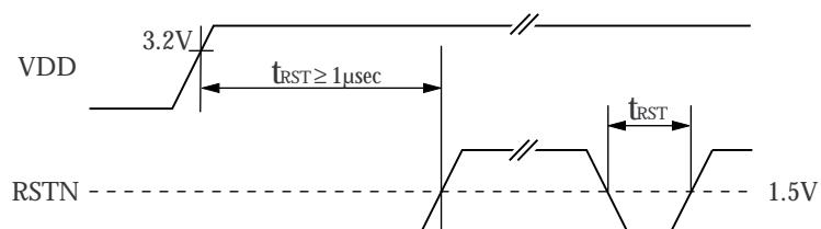
RSTN should be set LOW at power-ON and after reacquiring synchronization. Note that if RSTN is LOW for longer than  $1\mu\text{s}$ , a through-current flows in the internal dynamic circuits because the internal clock is stopped. The through-current has no rated value, so the reset pulse should be kept as short as possible at all times other than at power-ON.
