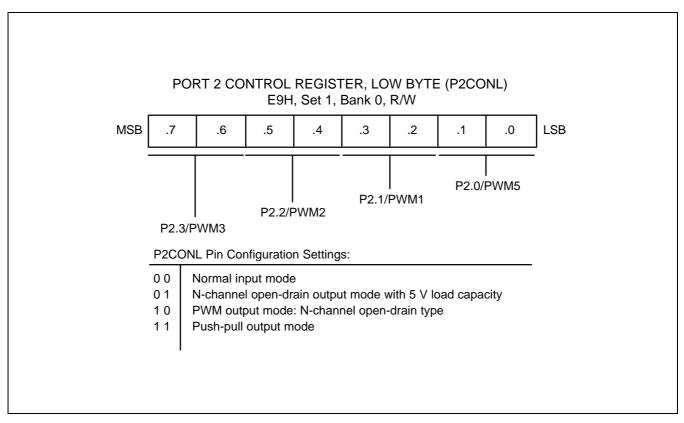
Figure 9-7. Port 2 Low-Byte Control Register (P2CONL)
