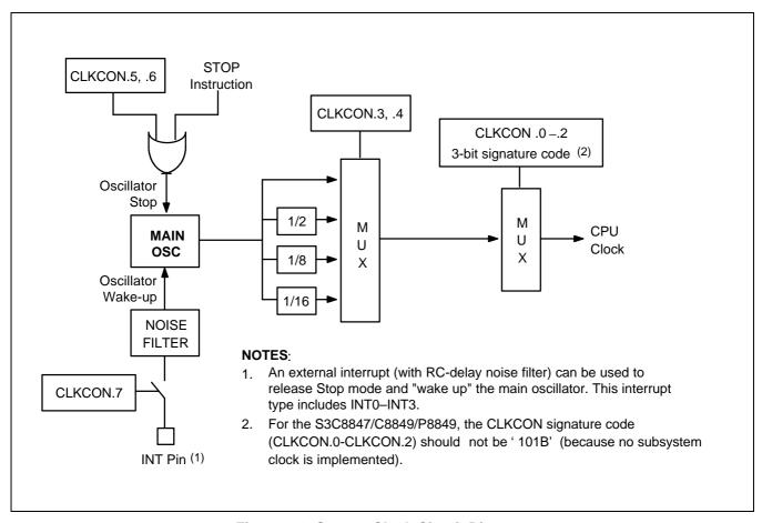
Figure 7-2. System Clock Circuit Diagram
