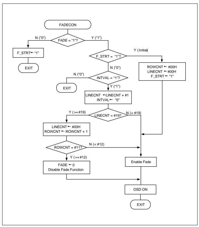
Figure 13-23. Decision Flowchart for Fade Function Programming Tip
