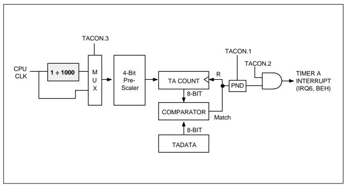
Figure 11-1. Timer A Block Diagram
