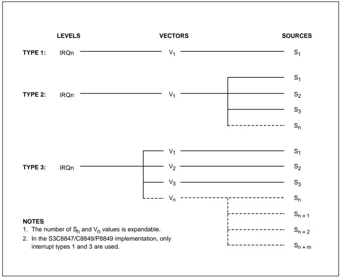
Figure 5-1. S3C8-Series Interrupt Types
