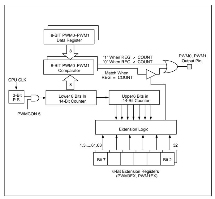
Figure 12-5. Block Diagram for PWM0 and PWM1
