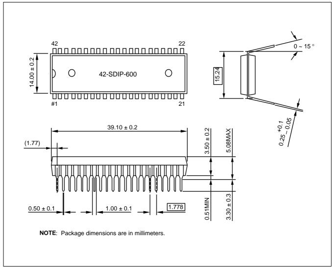
Figure 16-1. 42-Pin SDIP Package Mechanical Data (42-SDIP-600)
