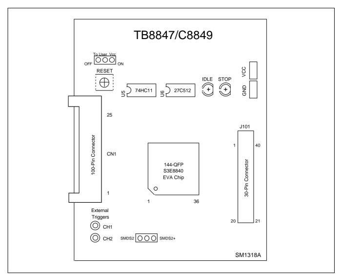
Figure 18-2. TB8847/8849 Target Board Configuration
