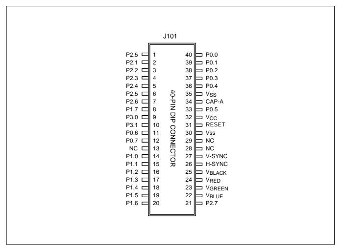
Figure 18-3. 40-Pin DIP Connector J101 for TB8847/8849
