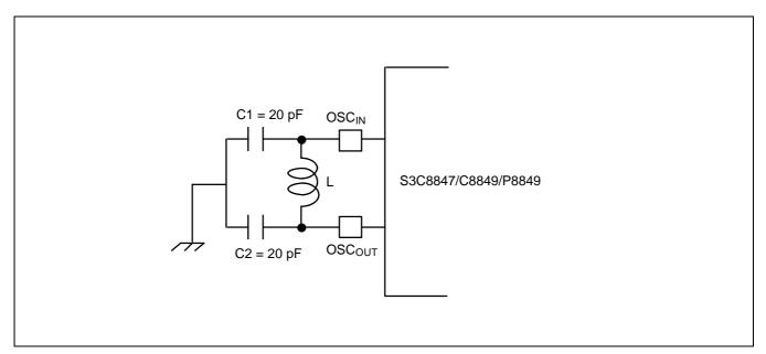
Figure 7-4. L-C Oscillator Circuit for OSD
