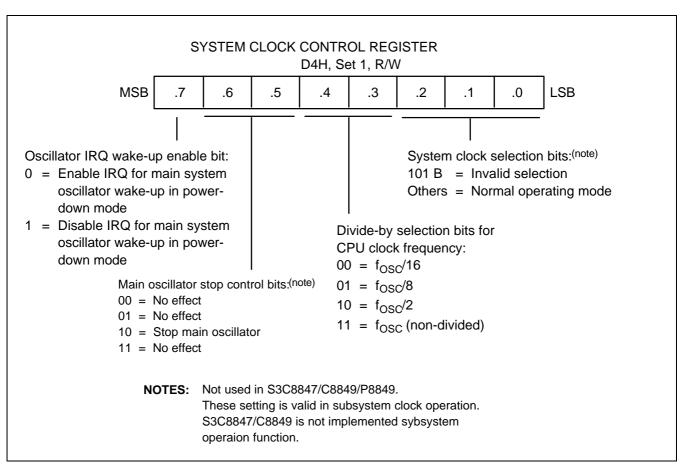
Figure 7-3. System Clock Control Register (CLKCON)
