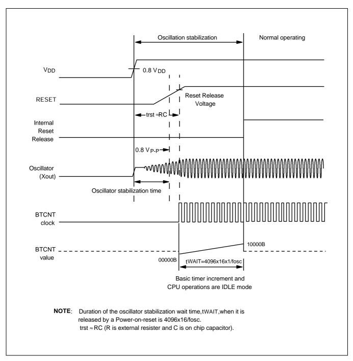
Figure 10-2. Oscillation Stabilization Time on RESET
