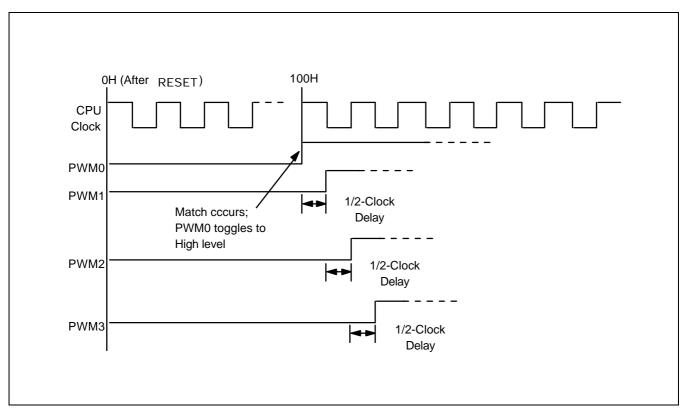
Figure 12-4. PWM Clock to PWM2-PWM5 Output Delays
