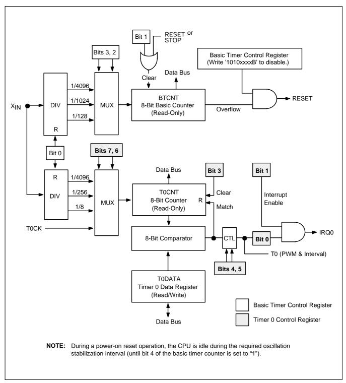
Figure 10-7. Basic Timer and Timer 0 Block Diagram
