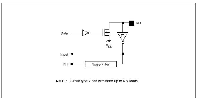
Figure 1-9. Pin Circuit Type 7 (P1.0–P1.3, INT0–INT3)
