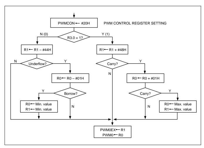
Figure 12-6. Decision Flowchart for PWM0 Programming Tip
