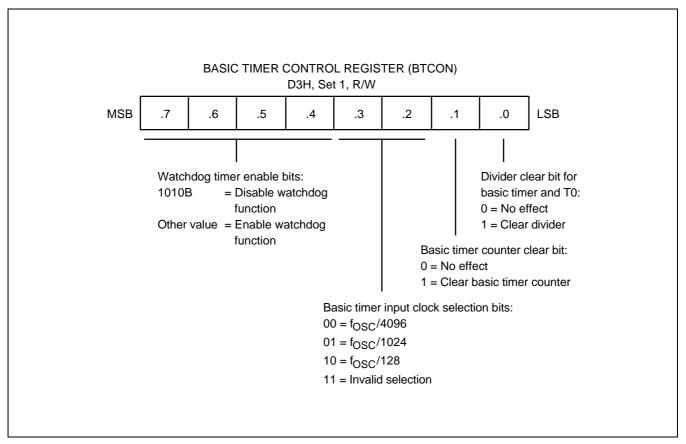
Figure 10-1. Basic Timer Control Register (BTCON)
