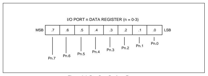
Figure 9-1. Port Data Register Format
