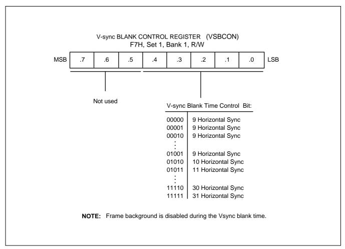
Figure 13-19. V-sync Blank Control Register (VSBCON)
