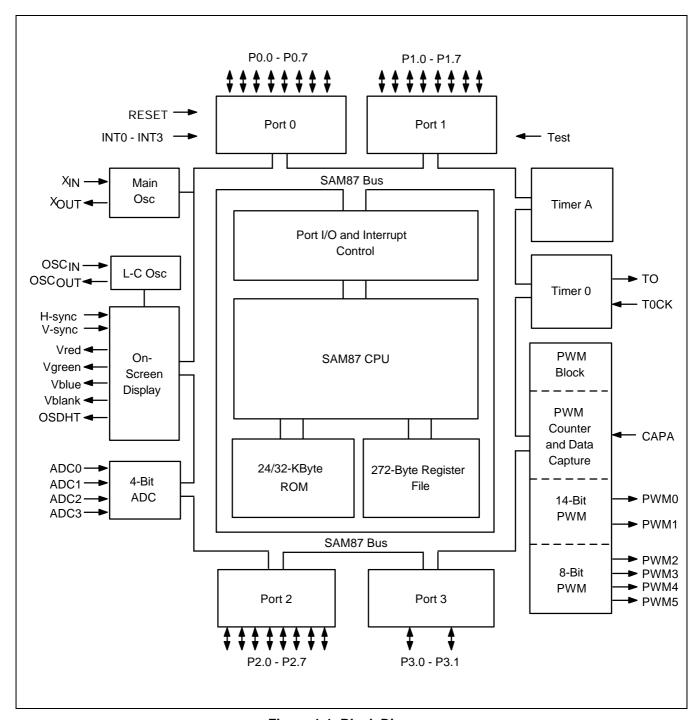
Figure 1-1. Block Diagram
