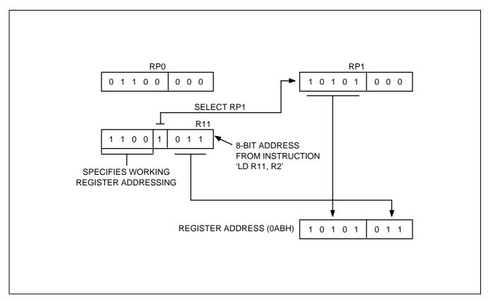
Figure 2-15. 8-Bit Working Register Addressing Example
