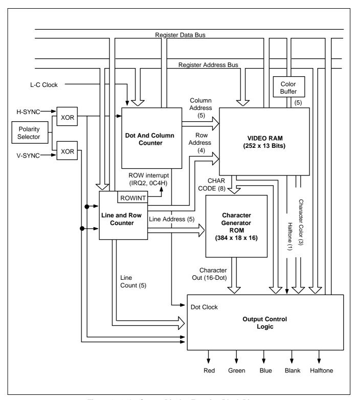
Figure 13-1. On-Screen Display Function Block Diagram
