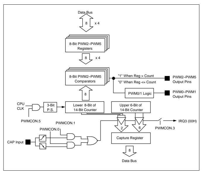
Figure 12-2. Block Diagram for PWM2-PWM5
