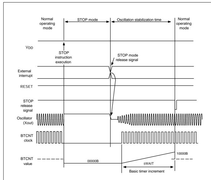
**NOTE:** Duration of the oscillator stabilization wait time, tWAIT, it is released by an interrupt is determined by the setting in basic timer control register, BTCON.
