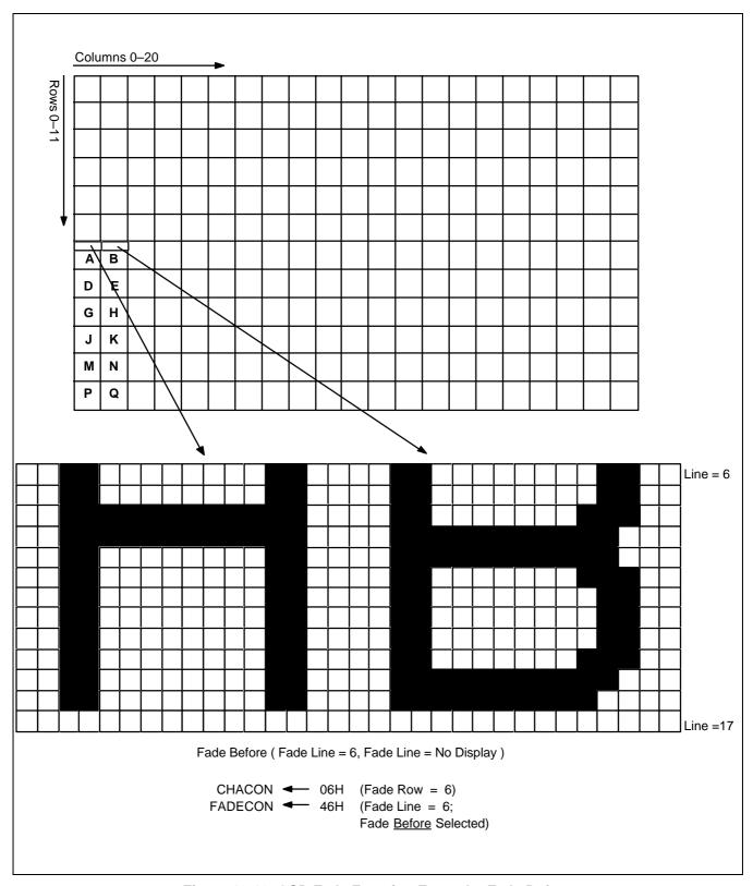
Figure 13-10. OSD Fade Function Example: Fade Before
