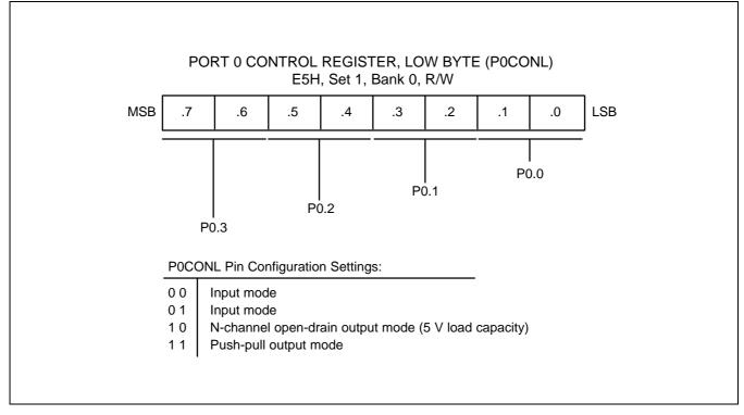
Figure 9-3. Port 0 Low-Byte Control Register (P0CONL)
