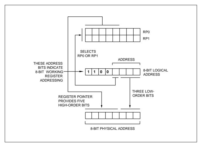
Figure 2-14. 8-Bit Working Register Addressing
