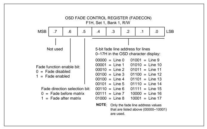
Figure 13-7. OSD Fade Control Register (FADECON)
