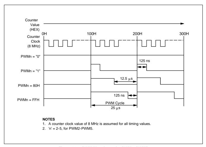
Figure 12-3. PWM Waveforms for PWM2-PWM5
