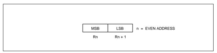
Figure 2-9. 16-Bit Register Pairs
