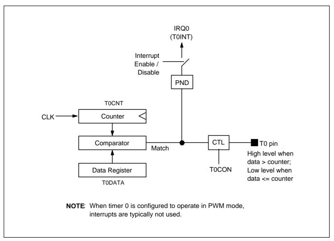
Figure 10-6. Timer 0 Function Diagram (PWM Mode)
