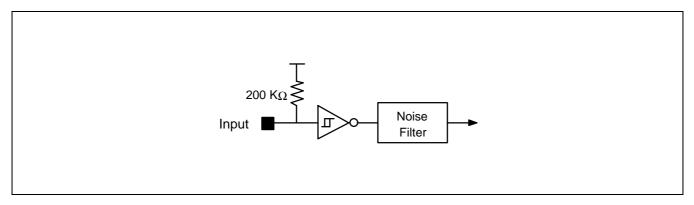
Figure 1-10. Pin Circuit Type 8 (RESET)
