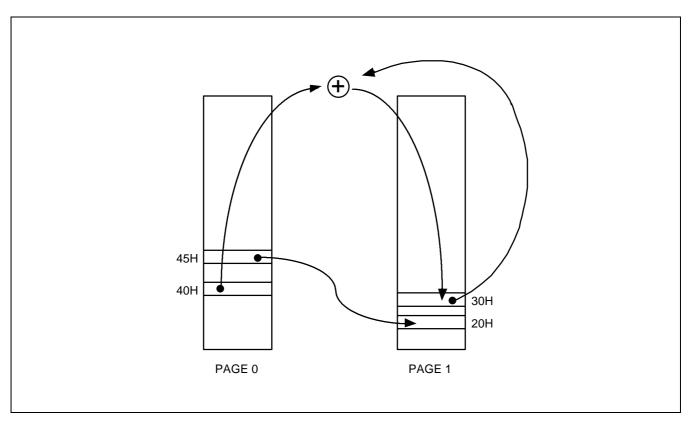
Figure 2-4. Programming Tip Example for Inter-Page Data Operations
