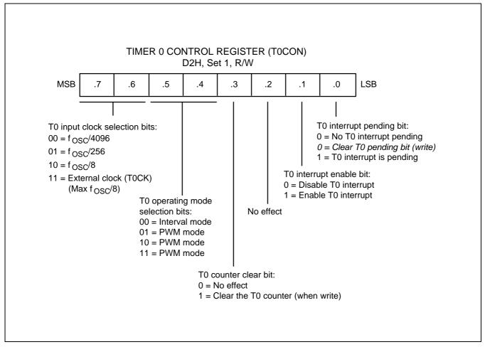
Figure 10-4. Timer 0 Control Register (T0CON)
