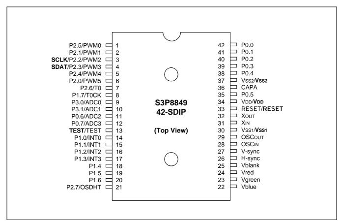
Figure 17-1. S3P8849 Pin Assignment (42-SDIP)
