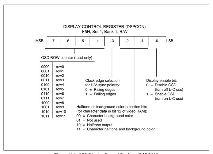
Figure 13-3. OSD Display Control Register (DSPCON)
