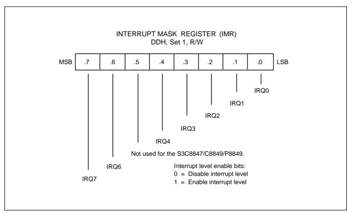
Figure 5-6. Interrupt Mask Register (IMR)
