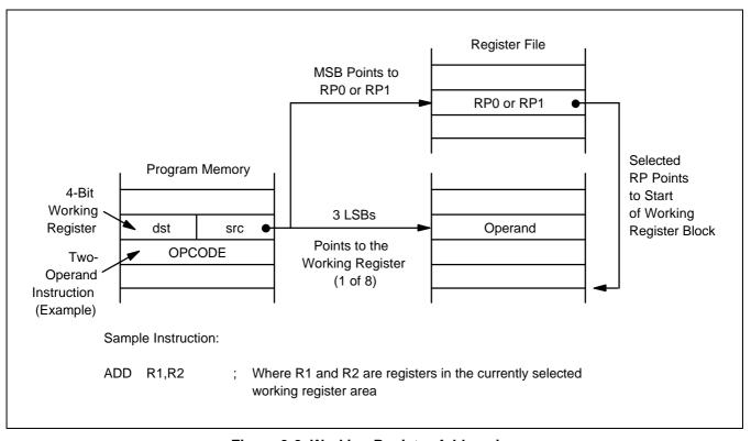
Figure 3-2. Working Register Addressing
