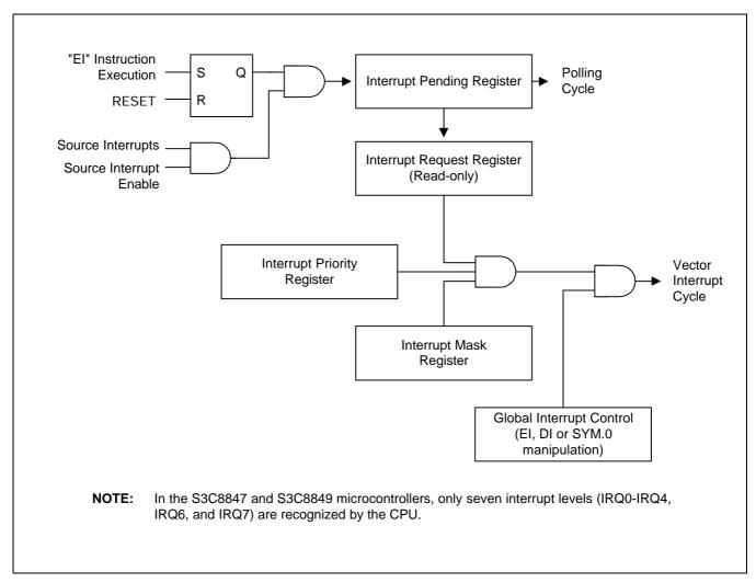
Figure 5-4. Interrupt Function Diagram
