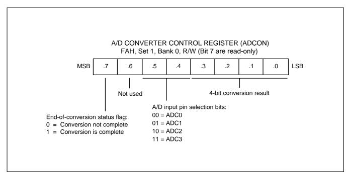
Figure 14-2. A/D Converter Control Register (ADCON)
