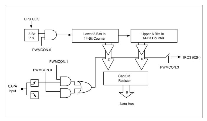
Figure 12-7. Block Diagram for Capture A
