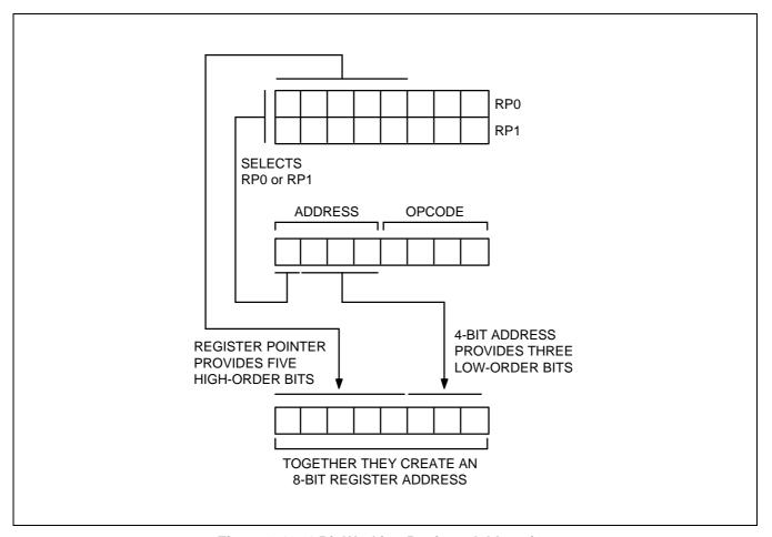
Figure 2-12. 4-Bit Working Register Addressing
