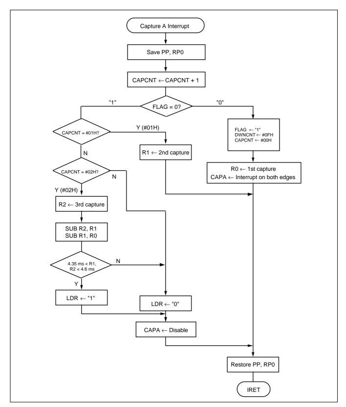
Figure 12-9. Decision Flowchart for Capture A Interrupt
