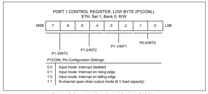
Figure 9-5. Port 1 Low-Byte Control Register (P1CONL)
