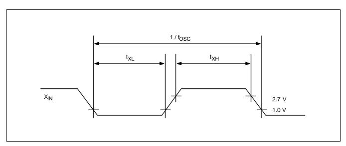
Figure 15-3. Clock Timing Measurement Points for  $\mathbf{X}_{\mathrm{IN}}$
