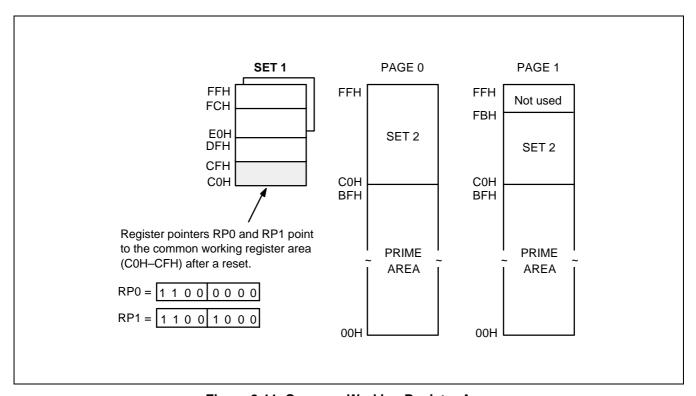
Figure 2-11. Common Working Register Area
