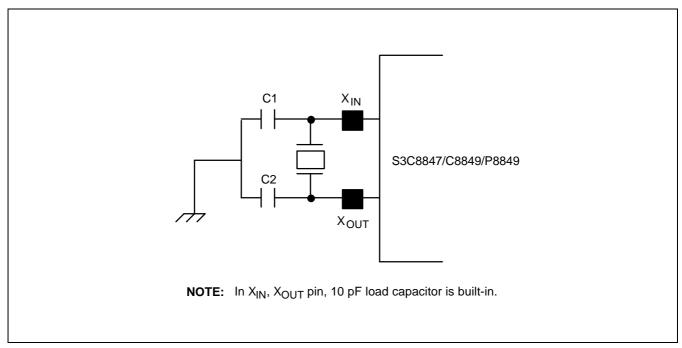
Figure 7-1. Main Oscillator Circuit (External Crystal or Ceramic Resonator)
