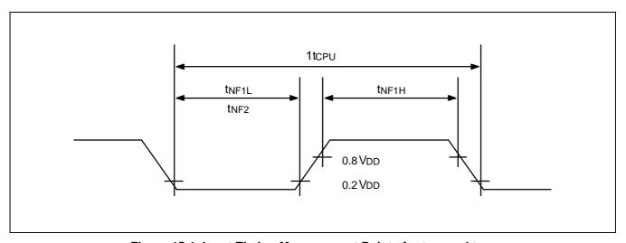
Figure 15-1. Input Timing Measurement Points for  $t_{\rm NF1}$  and  $t_{\rm NF2}$
