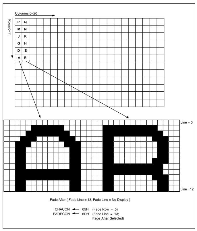
Figure 13-9. OSD Fade Function Example: Fade After
