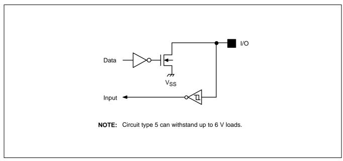
Figure 1-7. Pin Circuit Type 5 (P1.4–P1.5)
