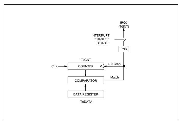
Figure 10-5. Timer 0 Function Diagram (Interval Timer Mode)
