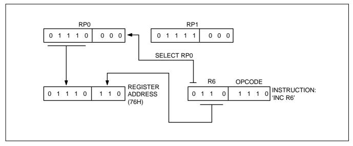
Figure 2-13. 4-Bit Working Register Addressing Example
