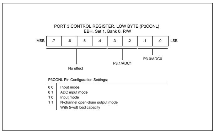
Figure 9-8. Port 3 Low-Byte Control Register (P3CONL)
