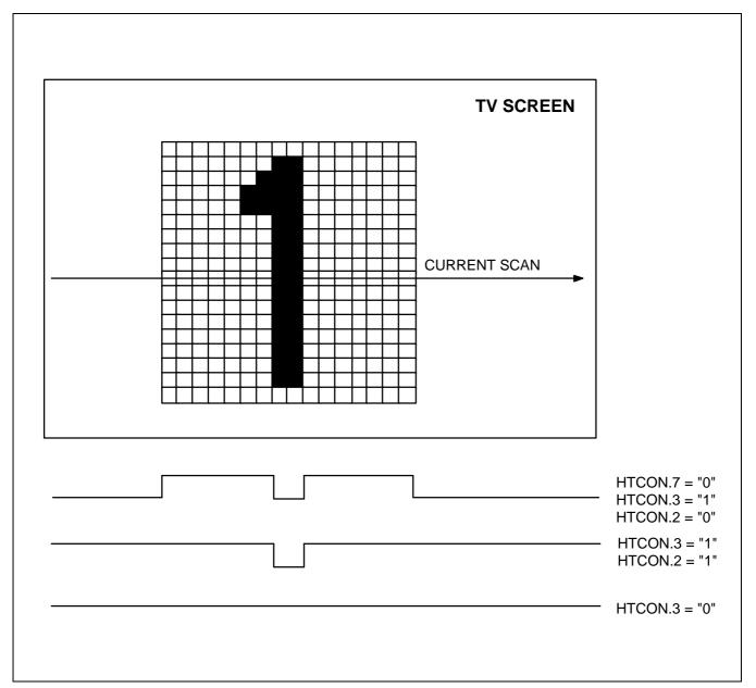
Figure 13-21. Halftone Control Signal Output Options
