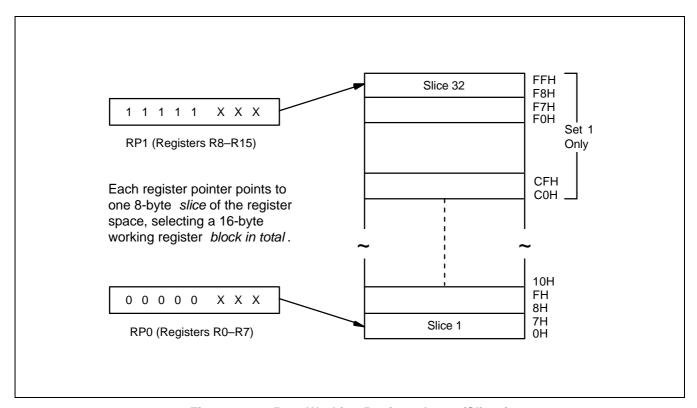
Figure 2-6. 8-Byte Working Register Areas (Slices)
