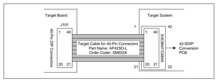
Figure 18-4. S3C8847/C8849 Probe Adapter for 42-SDIP Package
