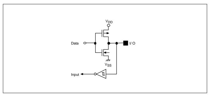
Figure 1-5. Pin Circuit Type 3 (P0.4–P0.5, P1.6–P1.7, T0CK)
