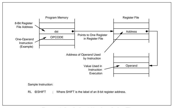
Figure 3-3. Indirect Register Addressing to Register File
