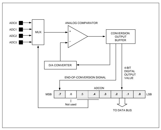
Figure 14-1. A/D Converter Functional Block Diagram
