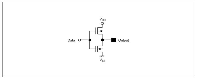
Figure 1-6. Pin Circuit Type 4 (Vblue, Vgreen, Vred, Vblank)
