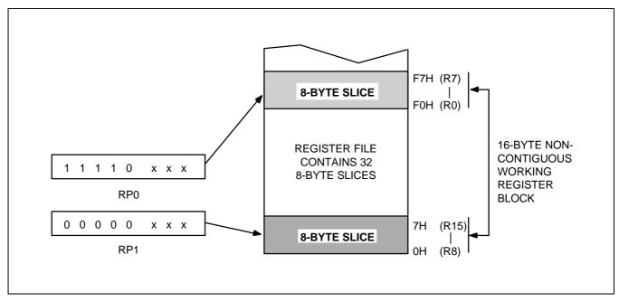
Figure 2-8. Non-Contiguous 16-Byte Working Register Block
