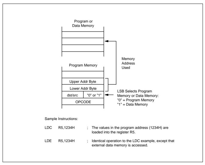
Figure 3-10. Direct Addressing for Load Instructions
