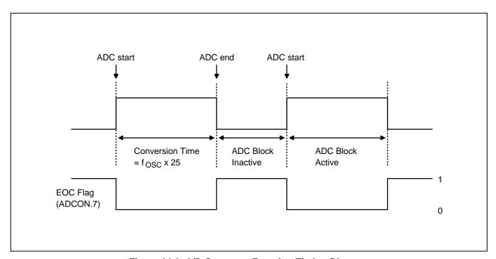
Figure 14-3. A/D Converter Function Timing Diagram
