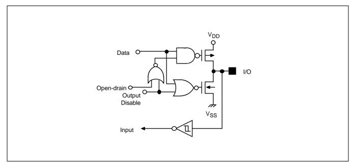
Figure 1-4. Pin Circuit Type 2 (P2.0–P2.7, P0.0–P0.3, PWM0–PWM5, T0, OSDHT)
