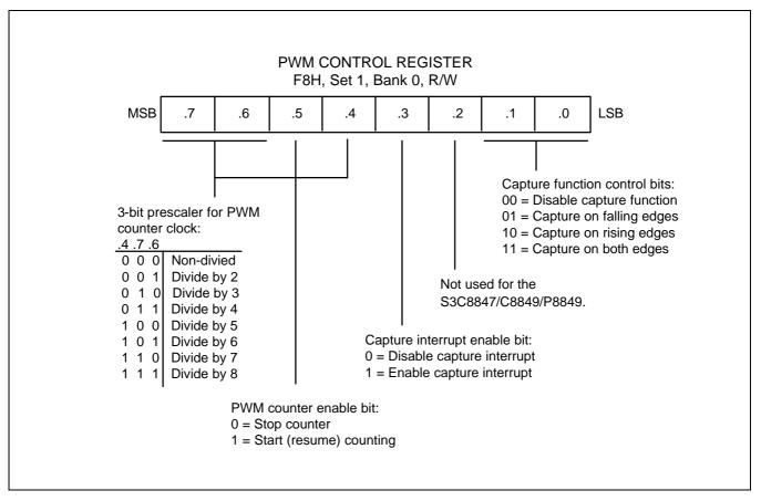
Figure 12-1. PWM Control Register (PWMCON)
