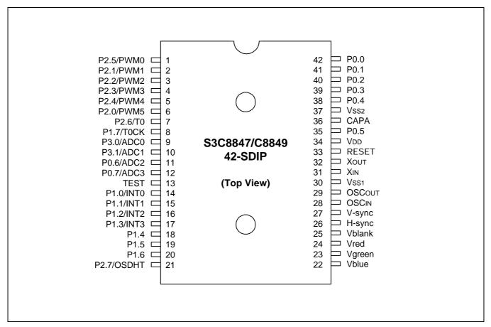
Figure 1-2. S3C8847/C8849/P8849 Pin Assignment Diagram
