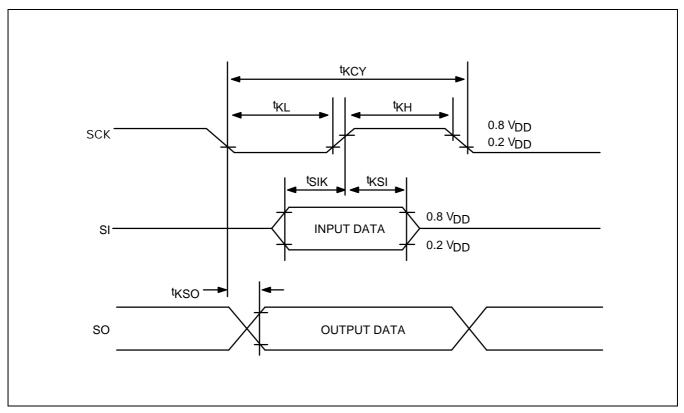
Figure 14–10. Serial Data Transfer Timing
