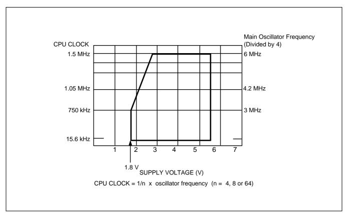
Figure 16–2. Standard Operating Voltage Range
