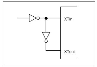
Figure 6-6. External Oscillator (fxt)
