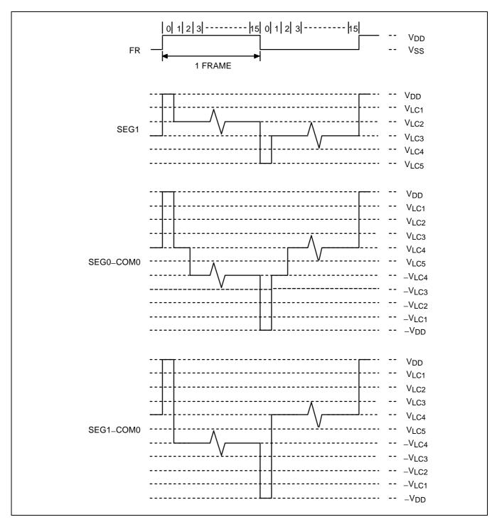
Figure 12-6. LCD Signal Waveforms (1/16 Duty, 1/5 Bias) (Continued)
