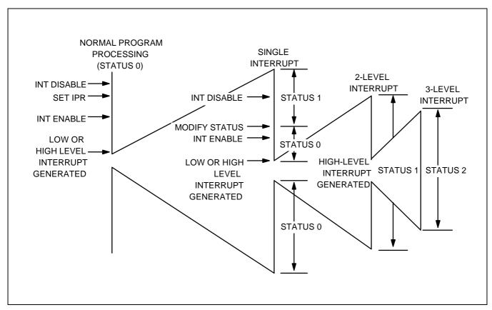
Figure 7-4. Multi-Level Interrupt Handling
