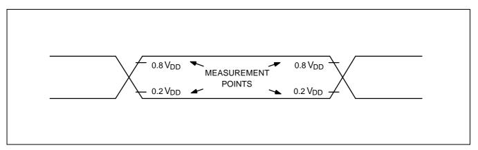
Figure 14–4. A.C. Timing Measurement Points (Except for X<sub>in</sub> and XT<sub>in</sub>)
