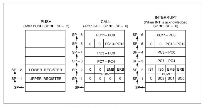
Figure 2–7. Push-Type Stack Operations
