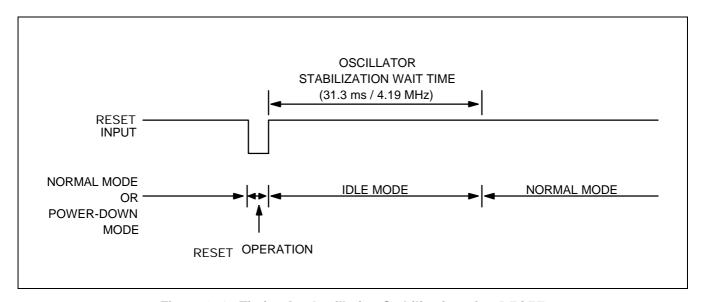
Figure 9-1. Timing for Oscillation Stabilization after RESET
