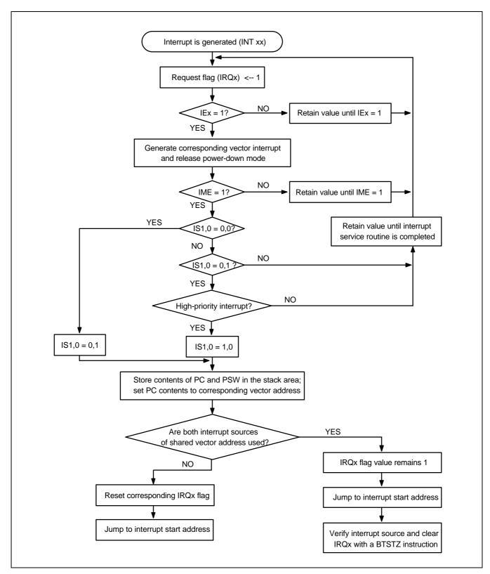
Figure 7-1. Interrupt Execution Flowchart
