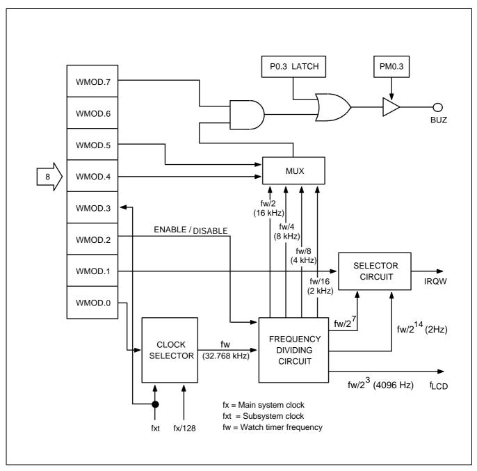
Figure 11-6. Watch Timer Circuit Diagram
