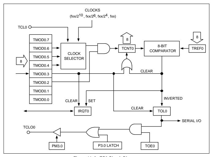
Figure 11-2. TC0 Circuit Diagram
