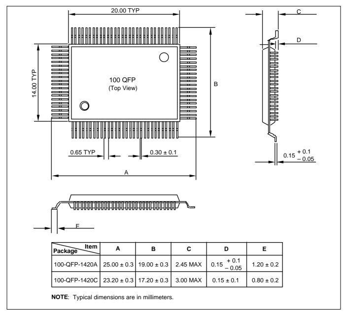
Figure 15-1. 100-QFP Package Dimensions
