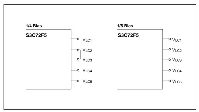
Figure 12-4. LCD Bias Circuit Connection
