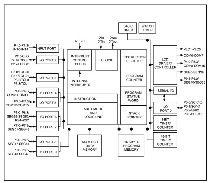
Figure 1-1. S3C72F5 Simplified Block Diagram
