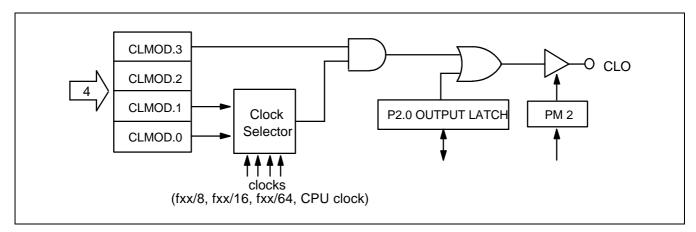
Figure 6-7. CLO Output Pin Circuit Diagram
