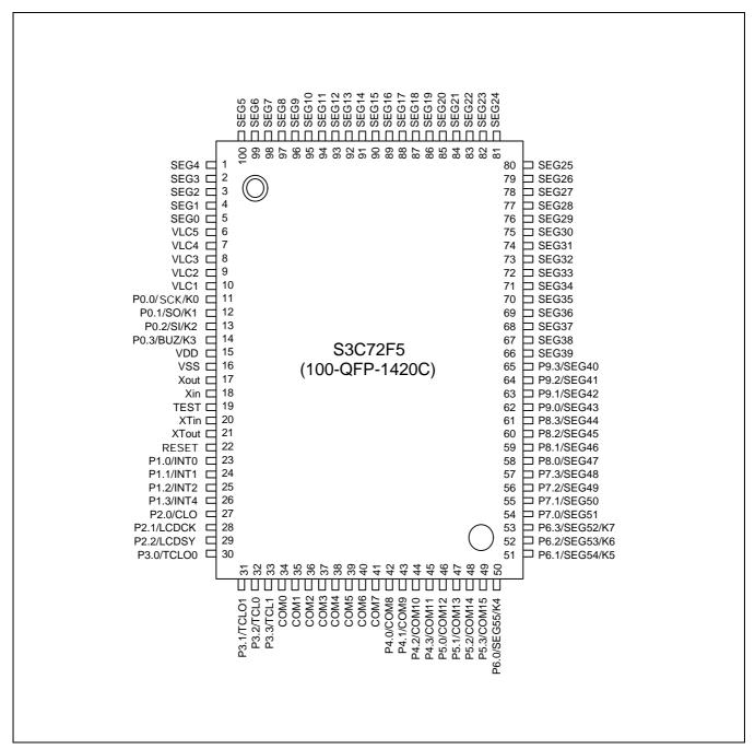
Figure 1-2. S3C72F5 100-QFP Pin Assignment Diagram
