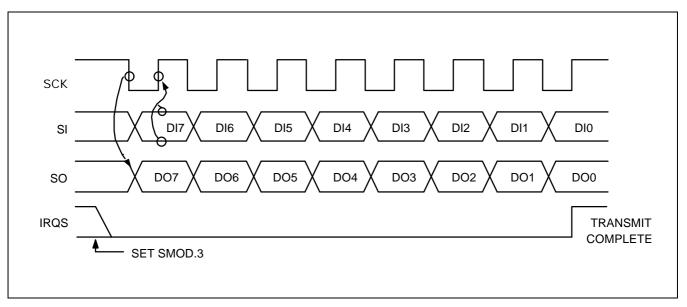
Figure 13–2. SIO Timing in Transmit/Receive Mode
