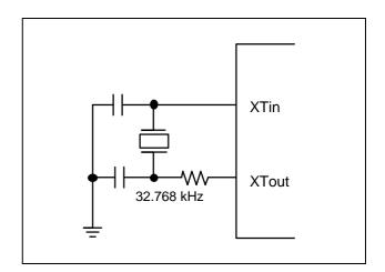
Figure 6-5. Crystal/Ceramic Oscillator (fxt)
