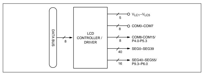
Figure 12-1. LCD Function Diagram
