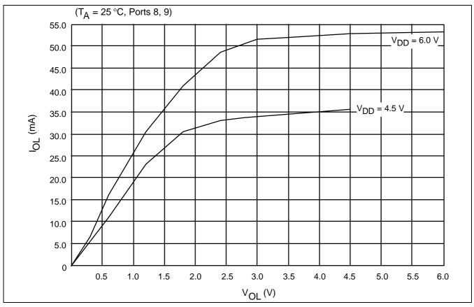
Figure 14-18. I<sub>OL</sub> VS. V<sub>OL</sub> (P8, 9)
