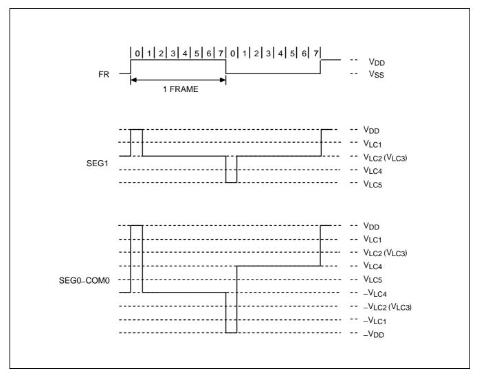
Figure 12-7. LCD Signal Waveforms (1/8 Duty, 1/4 Bias) (Continued)
