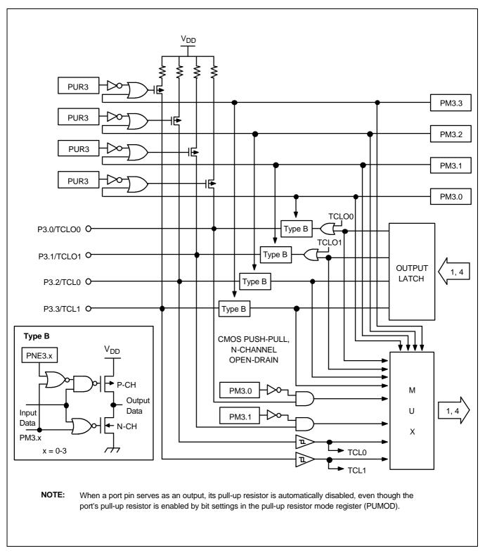
Figure 10-4. Port 3 Circuit Diagram
