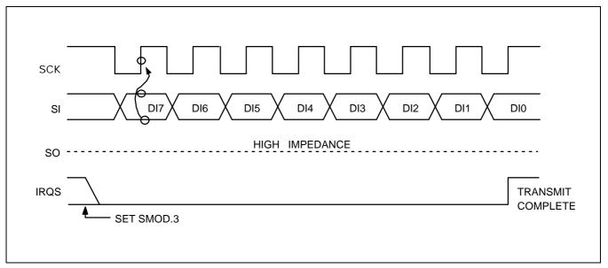
Figure 13-3. SIO Timing in Receive-Only Mode
