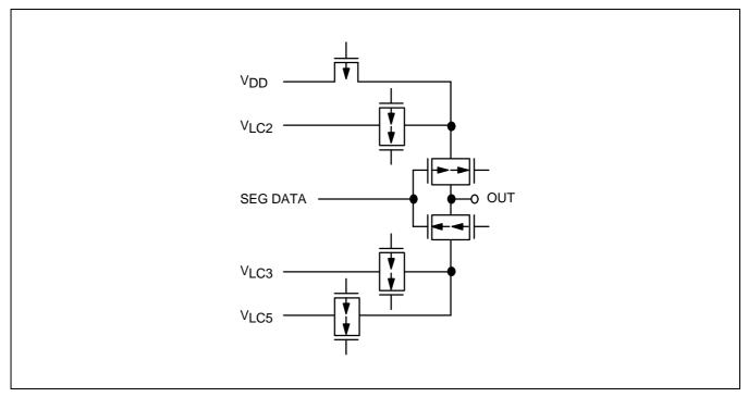
Figure 1-11. Pin Circuit Type H-15
