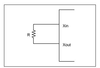
Figure 6-4. RC Oscillator (fx)
