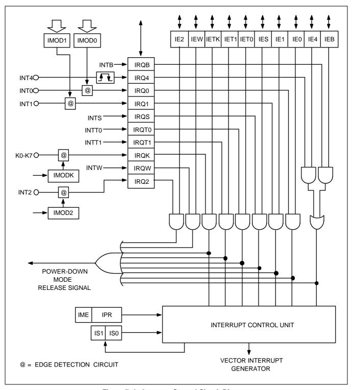
Figure 7–2. Interrupt Control Circuit Diagram
