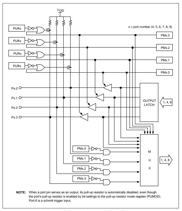
Figure 10-5. Ports 4, 5, 6, 7, 8, and 9 Circuit Diagram
