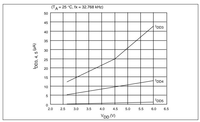
Figure 14–12.  $I_{DD3}$ ,  $I_{DD4}$ ,  $I_{DD5}$  VS.  $V_{DD}$
