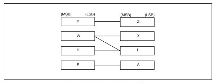
Figure 2-5. Register Pair Configuration
