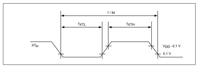
Figure 14–6. Clock Timing Measurement at XT<sub>in</sub>
