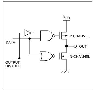
Figure 1-6. Pin Circuit Type C
