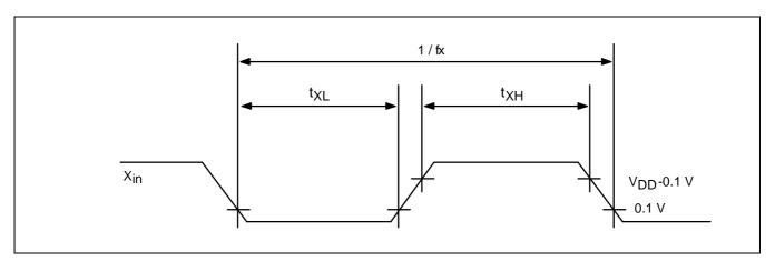
Figure 14–5. Clock Timing Measurement at Xin
