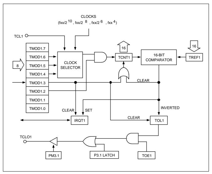
Figure 11-4. TC1 Circuit Diagram
