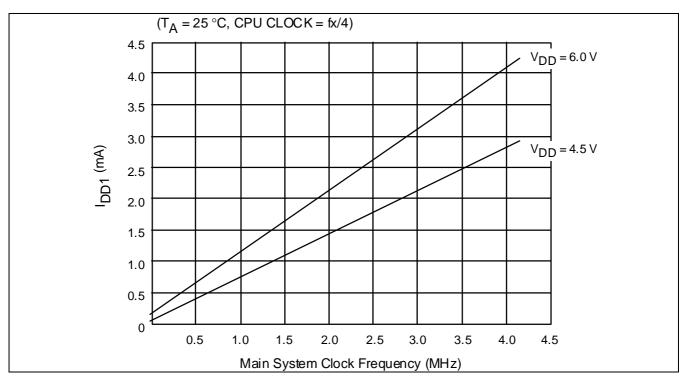
Figure 14–13. I<sub>DD1</sub> VS. Main System Clock Frequency
