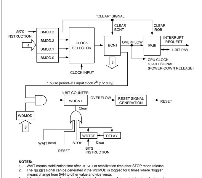
3. When the watchdog timer is enabled or the 3-bit counter of the watchdog timer is cleared to "0", the BCNT value is not cleared but increased continuously.
