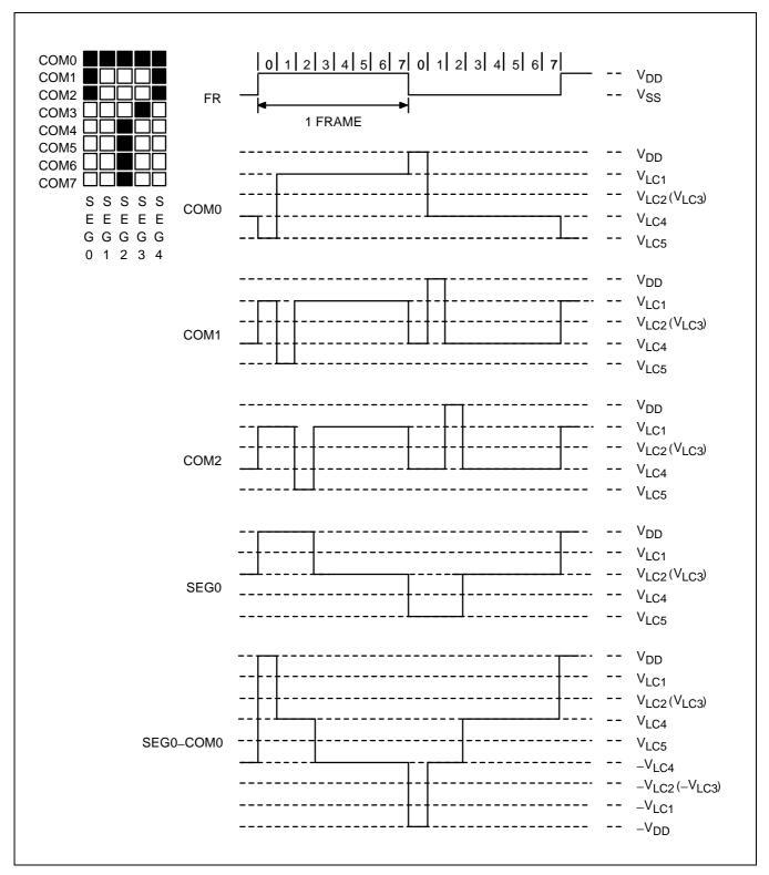
Figure 12-7. LCD Signal Waveforms (1/8 Duty, 1/4 Bias)
