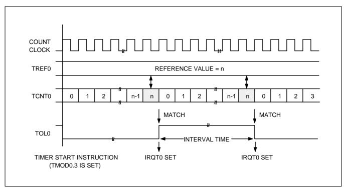
Figure 11-3. TC0 Timing Diagram
