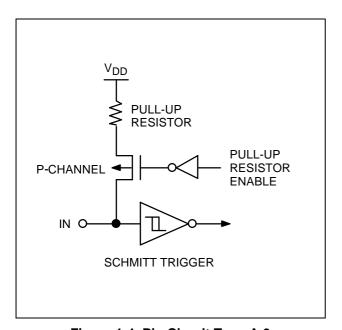
Figure 1-4. Pin Circuit Type A-3
