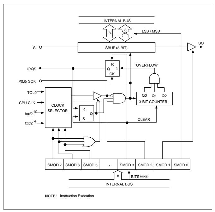
Figure 13-1. Serial I/O Interface Circuit Diagram
