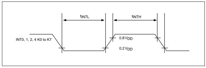
Figure 14–9. Input Timing for External Interrupts and Quasi-Interrupts
