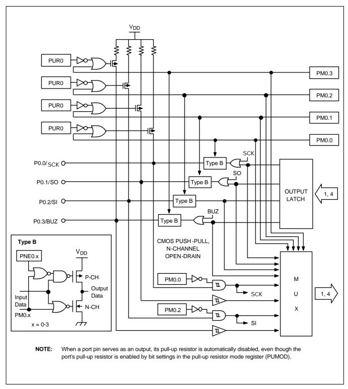
Figure 10–1. Port 0 Circuit Diagram
