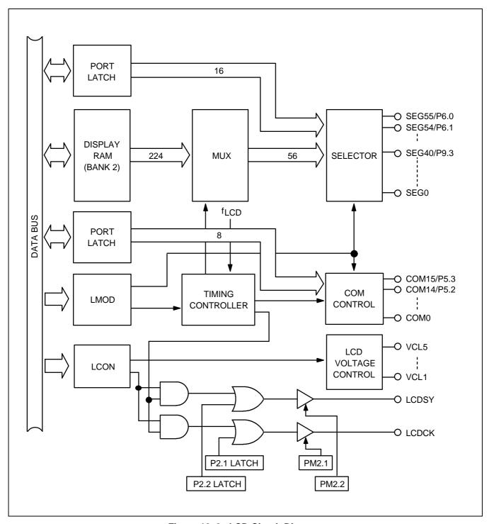
Figure 12-2. LCD Circuit Diagram
