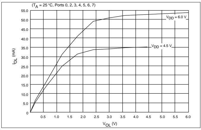
Figure 14-17. I<sub>OL</sub> VS. V<sub>OL</sub> (P0, 2, 3, 4, 5, 6, 7)
