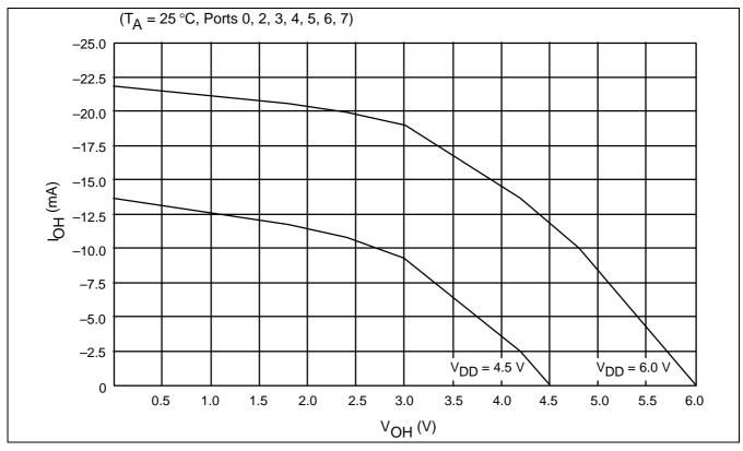
Figure 14-15. I<sub>OH</sub> VS. V<sub>OH</sub> (P0, 2, 3, 4, 5, 6, 7)
