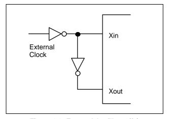
Figure 6-3. External Oscillator (fx)
