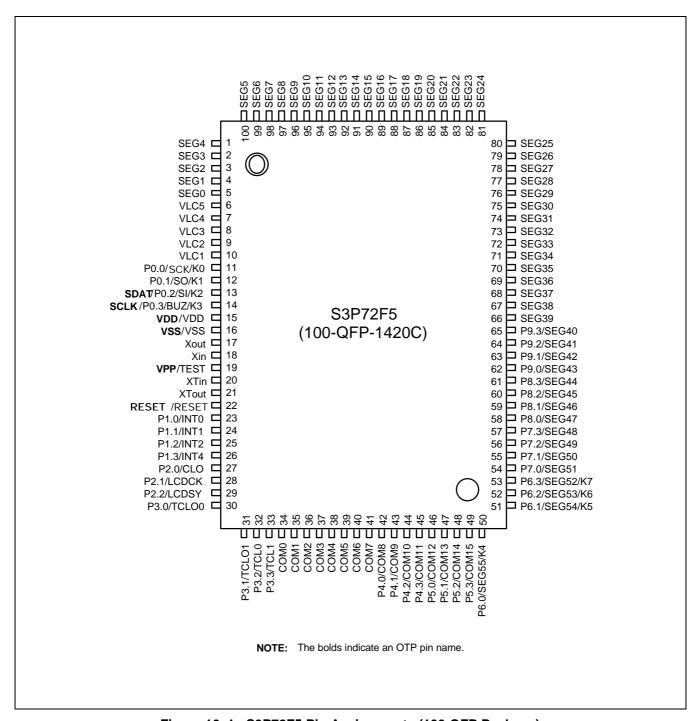
Figure 16-1. S3P72F5 Pin Assignments (100-QFP Package)
