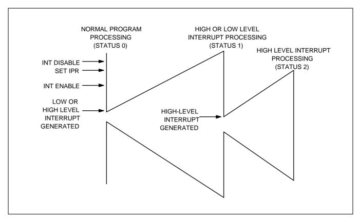
Figure 7–3. Two-Level Interrupt Handling
