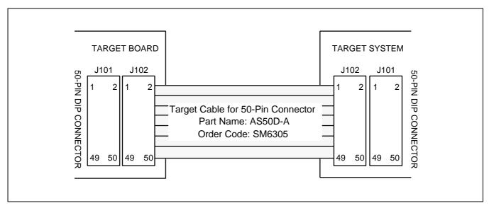
Figure 17-4. TB72F5 Adapter Cable for 100 QFP Package (S3C72F5)
