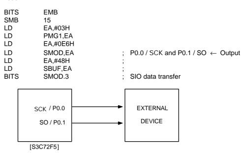
2. Use CPU clock to transfer and receive serial data at high speed:
