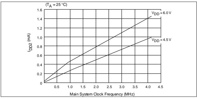
Figure 14-14. I<sub>DD2</sub> VS. Main System Clock Frequency
