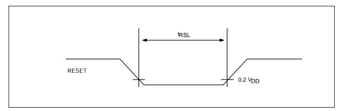
Figure 14-8. Input Timing for RESET Signal
