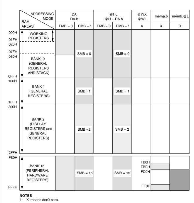
2. Blank columns indicate RAM areas that are not addressable, given the addressing method and enable memory bank (EMB) flag setting shown in the column headers.
