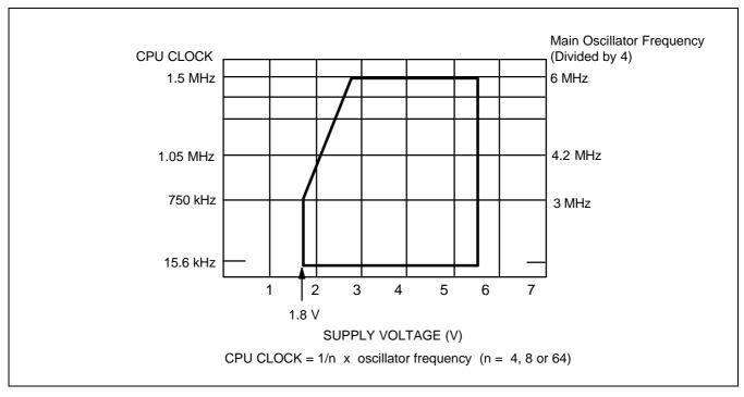
Figure 14–1. Standard Operating Voltage Range
