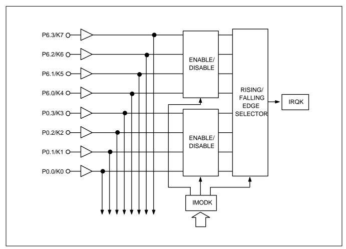
Figure 7–6. Circuit Diagram for INTK
