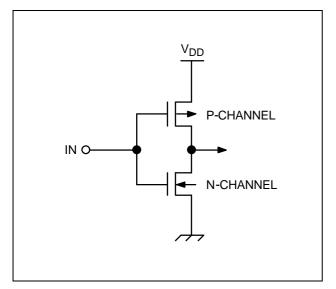
Figure 1-3. Pin Circuit Type A
