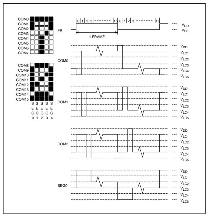
Figure 12-6. LCD Signal Waveforms (1/16 Duty, 1/5 Bias)
