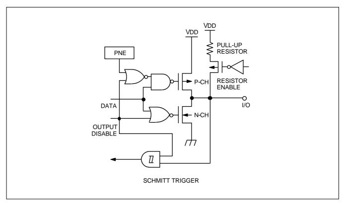
Figure 1-9. Pin Circuit Type E-2
