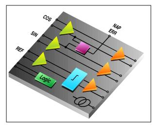
The sensoramplifier chip is intended for use in incremental position and angular measuring systems. It conditions the signals supplied by optical sensors.
