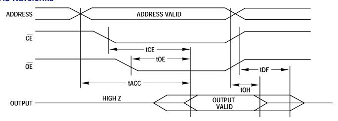
Notes:1. Timing measurement references are 1.5V. Input AC driving levels are 0V and 2.7V.
